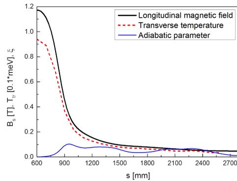
Figure 4: Variation of Longitudinal magnetic field  $B_s$ , transverse electron temperature  $T_{tr}$ , and adiabatic parameter  $\xi$  along the longitudinal coordinate  $s$ .
