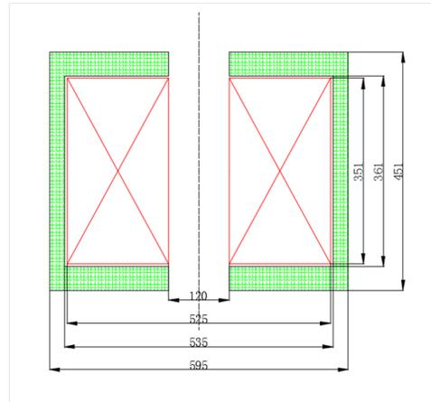
Figure 2: Cross section of the gun solenoid.
