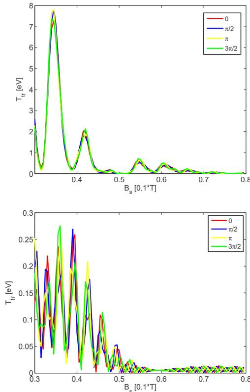
Figure 3: Dependence of transverse electron temperature upon the longitudinal magnetic field strength after toroid with (upper) and without (lower) the bending electro-static field. Electrons start from different initial phase advance of  $0, \pi/2, \pi, 3\pi/2$  in Larmor procession.
