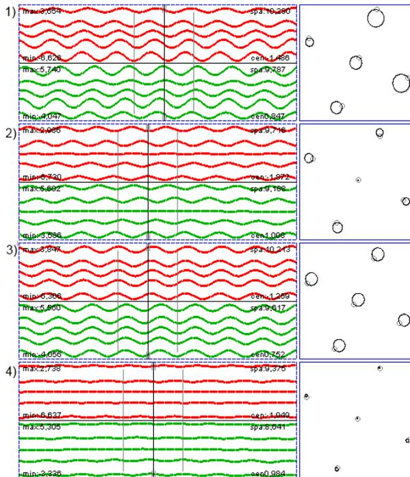
Figure 3: Trajectories in straight section. Red is projection in x, green is projection in y. First initial uncompensated beam, second larmor corrected, third galloping corrected, final larmor corrected again.
