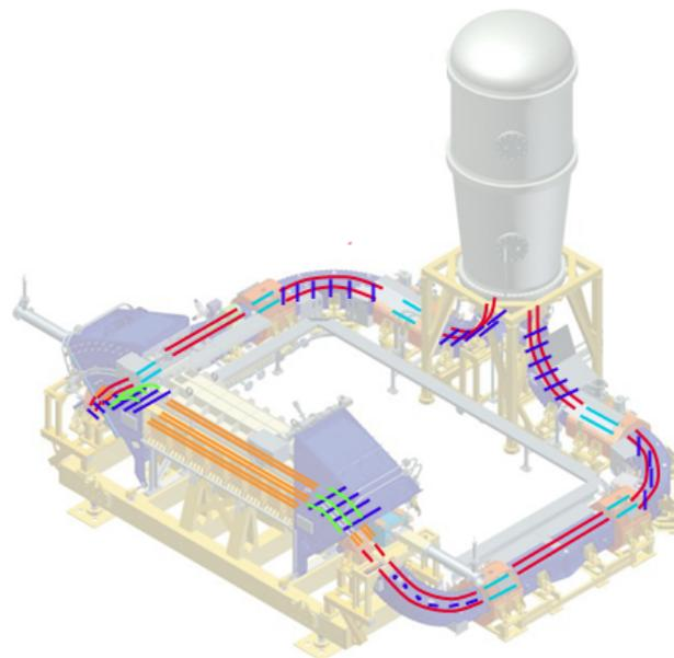
Figure 1: Image of the 2 MeV electron cooler. Equally colored symbolic field lines represent coils that share the same power supply. Orange: “Cooling section”, red: “Longitudinal field”, blue: “Bending field”, green: “Toroid 45° field”, and cyan: “Straight field”.
