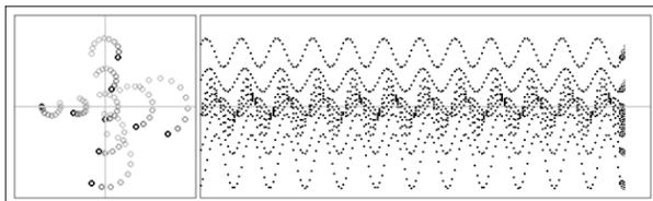
Figure 2: Trajectory cross sections to visualize the superposition of Larmor and galloping motion. Left in XY-Plane, right in YZ-Plane.
