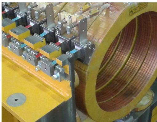
Figure 4: So-called pancake coils in cooling solenoid.
