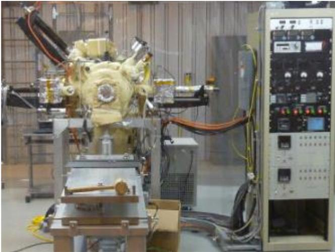
ERL Cathode deposition system at BLD912
