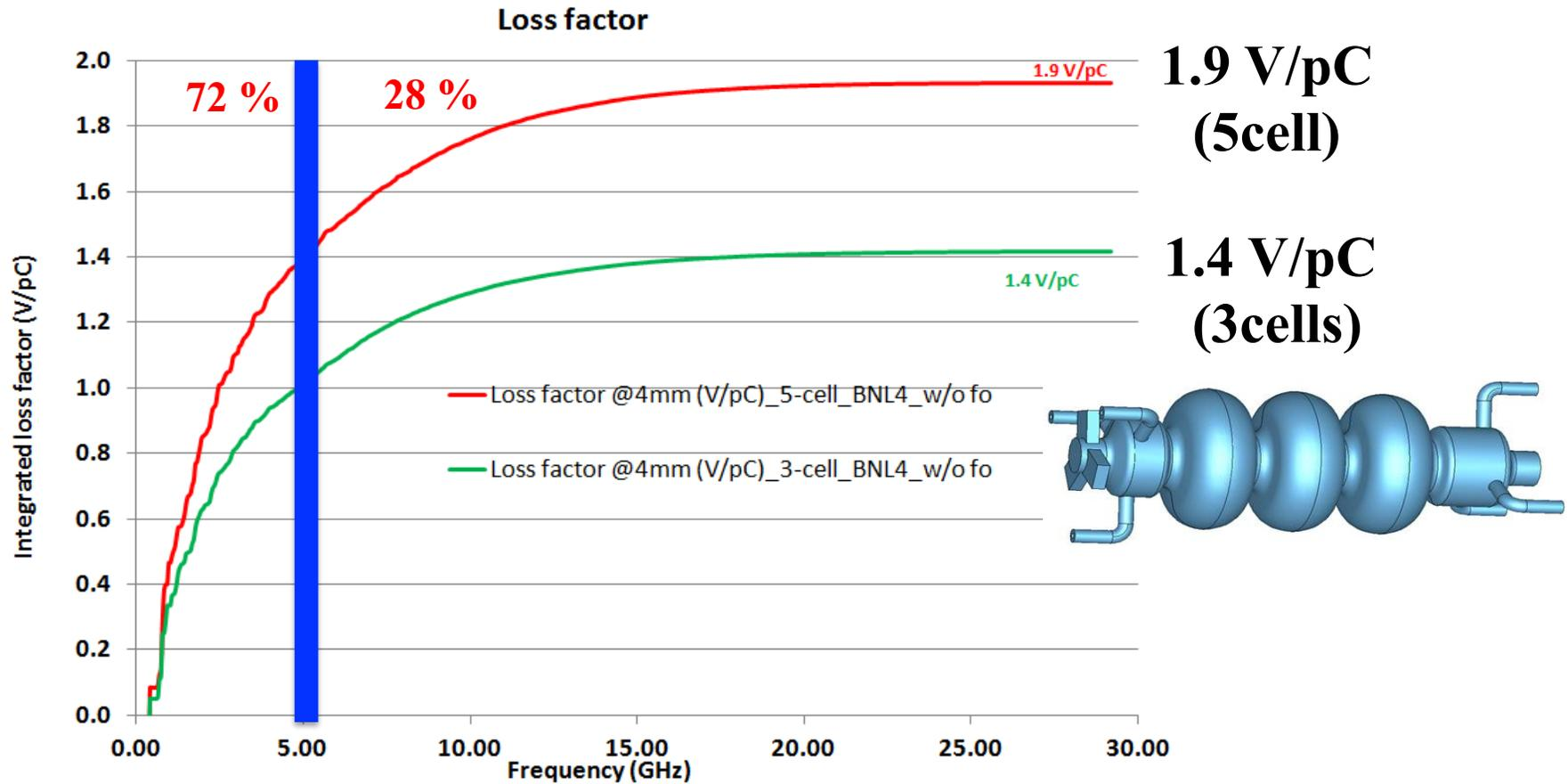
Fewer cells smaller loss factor per cavity.
