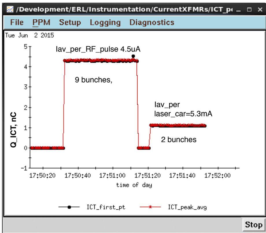
ICT signal for 9 pulses ( $4.4 \text{ nC} > 4 \text{ nC}$  ICT saturation)
