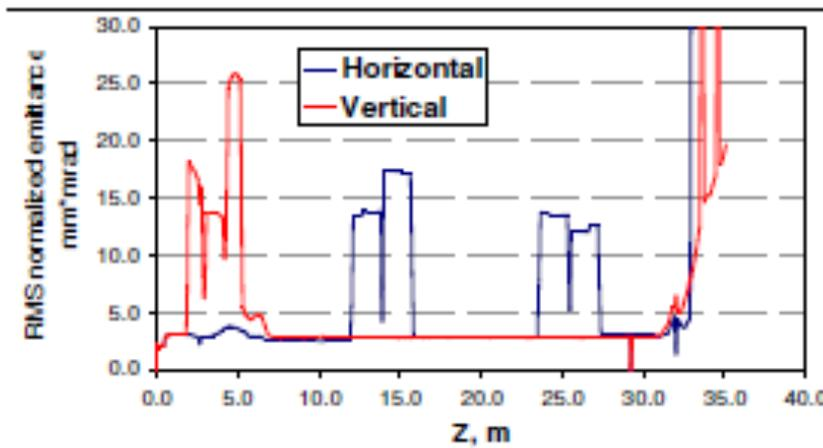
Transverse normalized emittances from cathode to dump  $Q=0.7$  nC (PARMELA simulation)
