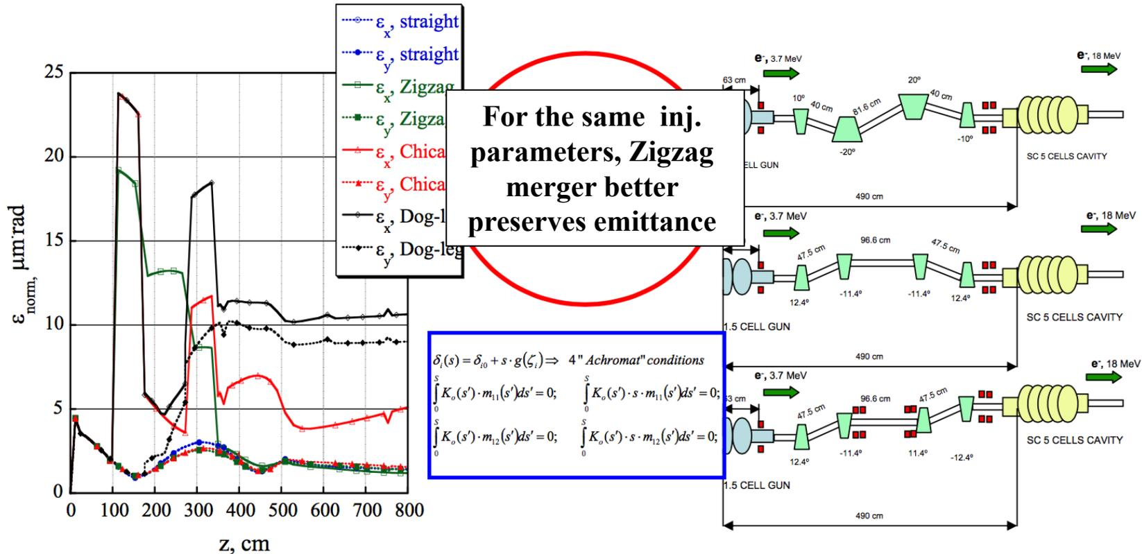
Evolution of horizontal and vertical normalized emittances in the four systems: the axially symmetric system (non shown), the Zigzag, the chicane and the Dog-leg.\*
