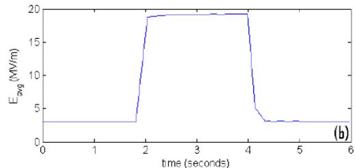
We find that by adopting a duty cycle of ~1:15 (on:off), we can safely turn the cavity up to an accelerating gradient of 18 MV/m. We demonstrated continuous running for 30 minutes with a pulse length of 2 seconds, and an off time of 30 seconds. During the “off” phase, the gradient is held at 3 MV/m. The longest pulse achieved before quenching was 5 seconds..
