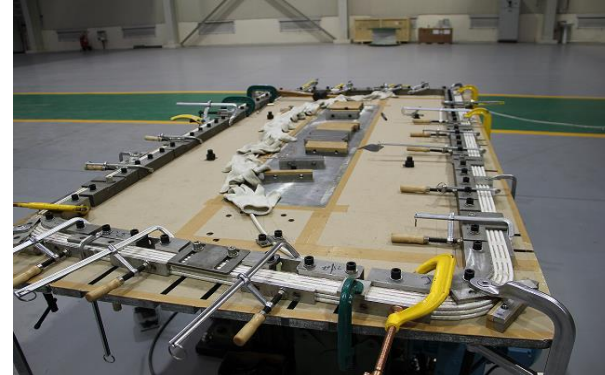
Fabrication of coil case
