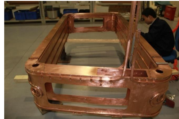
Fabrication of cryostat
