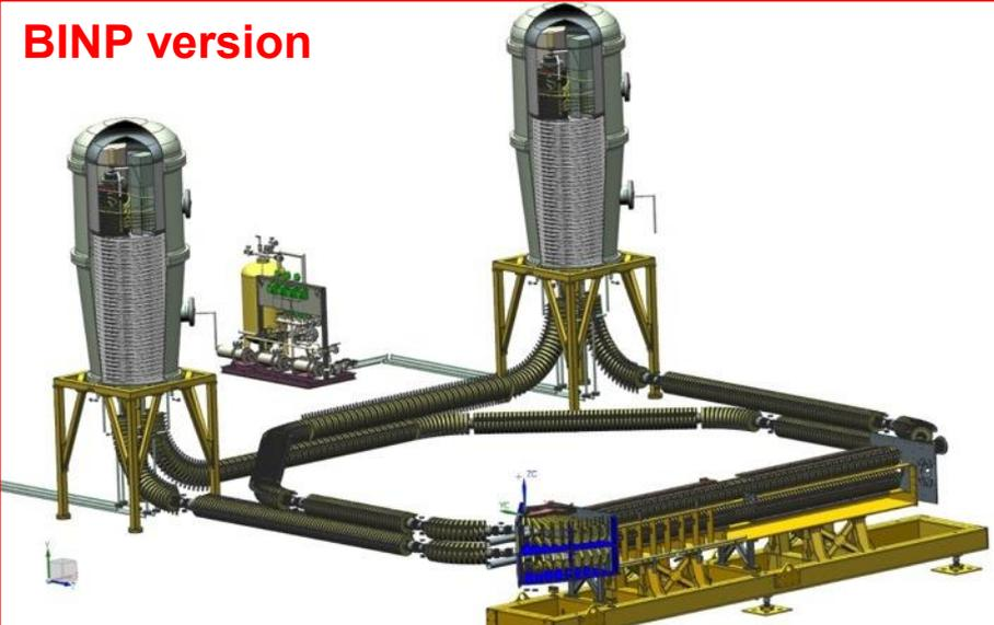
**Electron energy 0.5 ÷ 2.5 MeV, electron beam current 0.1 ÷ 1 A**
