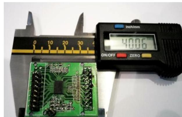
**Readout Electronics developed for TPC, TOF, and ECAL (64 ch, 13-bit, 65 MS/SPS)**
