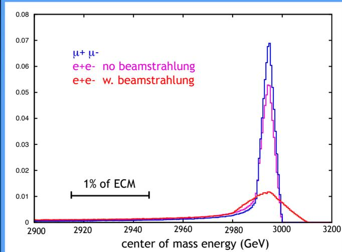
Effect of Beamstrahlung on CoM Energy Distribution at 3 TeV
