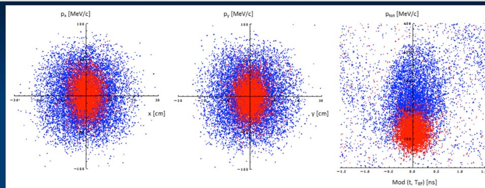
Initial 6D Cooling:  $\varepsilon_{6D} \ 60 \text{ cm}^3 \Rightarrow \sim 50 \text{ mm}^3$ ; Trans = 67%
