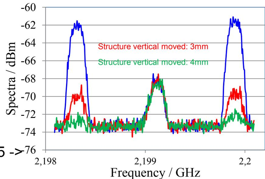
Betatron sidebands measured with the same structure (vertical tune close to 3.5  $\rightarrow$  bandoverlap)
