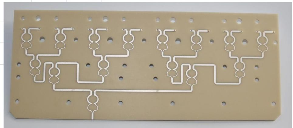
All  $\text{Al}_2\text{O}_3$  combiner-boards for main-system fabricated
