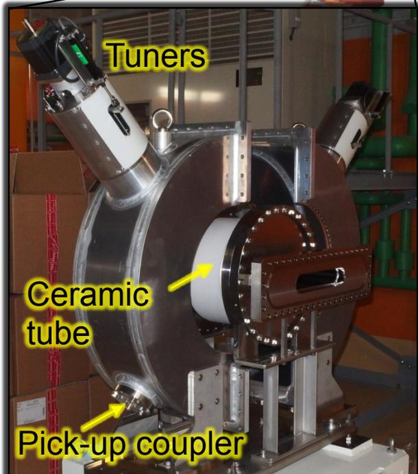
Resonance frequency : 173MHz (TM<sub>010</sub>)
