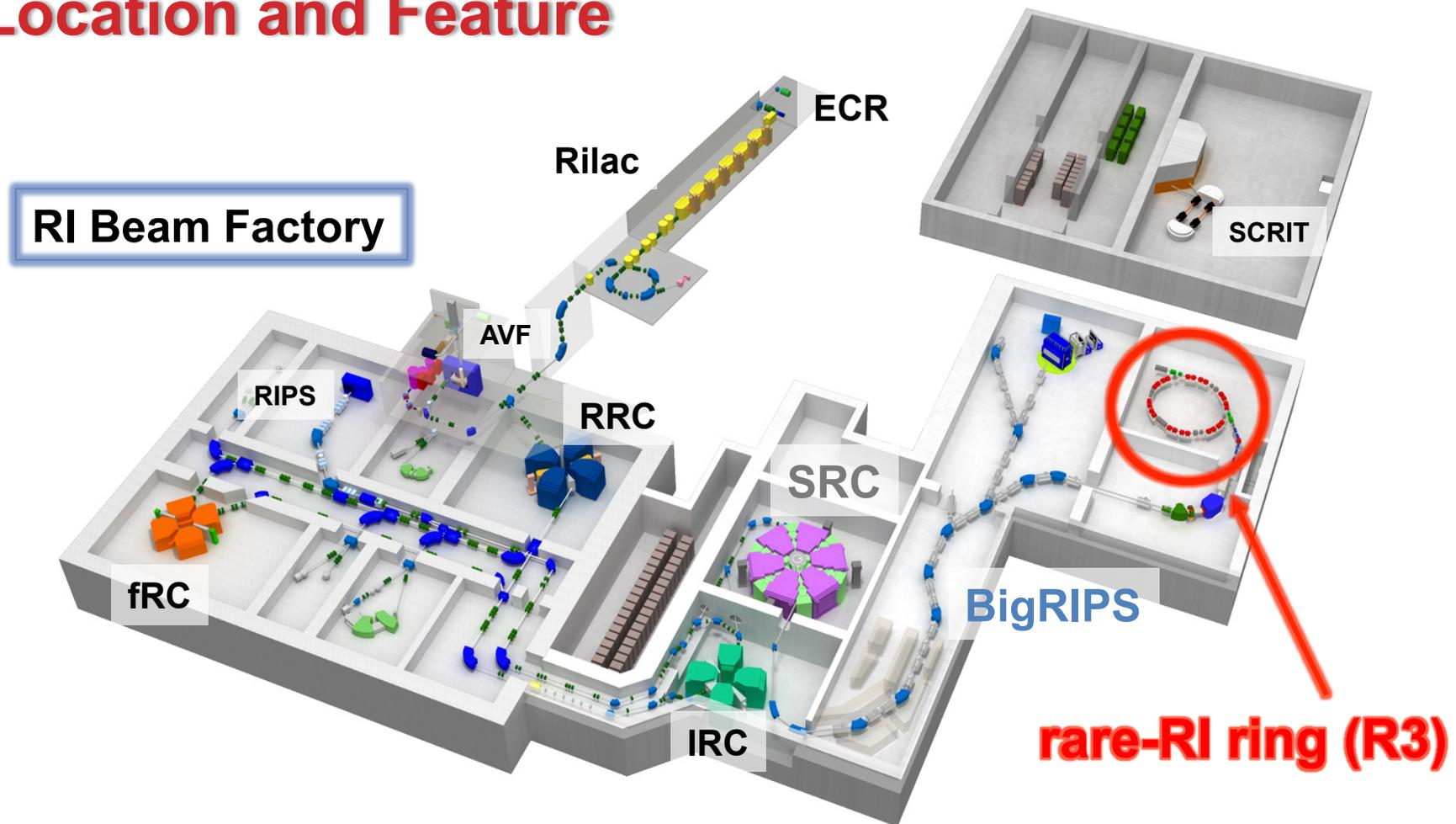
**A storage ring dedicated to mass measurements of exotic nuclei based on Isochronous Mass Spectrometry (IMS)**
