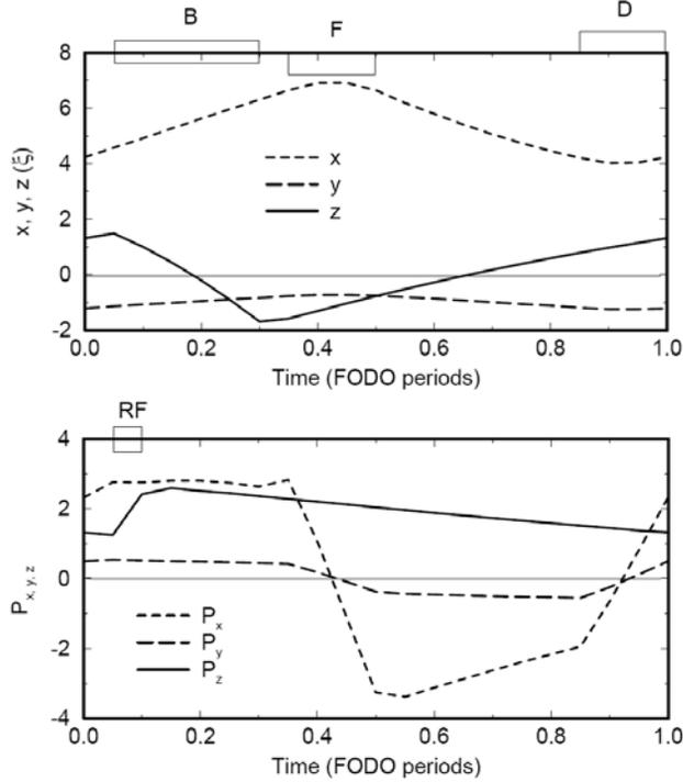
Figure 8: Particle trajectory of a bunched crystalline beam. The machine consists of 10 FODO cells with  $\nu_x=2.8$ ,  $\nu_y = 2.1$ , and  $\gamma = 1.4$ . Lattice components in each cell are displayed on the figure: B is a bending section, F and D are focusing and de-focusing quadrupoles, and RF is the bunching rf cavity.
