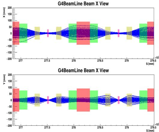
Figure 7: Last two cells for a beam emittance  $\epsilon_x = 126 \mu\text{m}$  rad and  $\epsilon_y = 622 \mu\text{m}$  rad through 210 cells with  $p = 622 \pm 2$  MeV/c. Red is RF. Green and yellow are quadrupoles.
