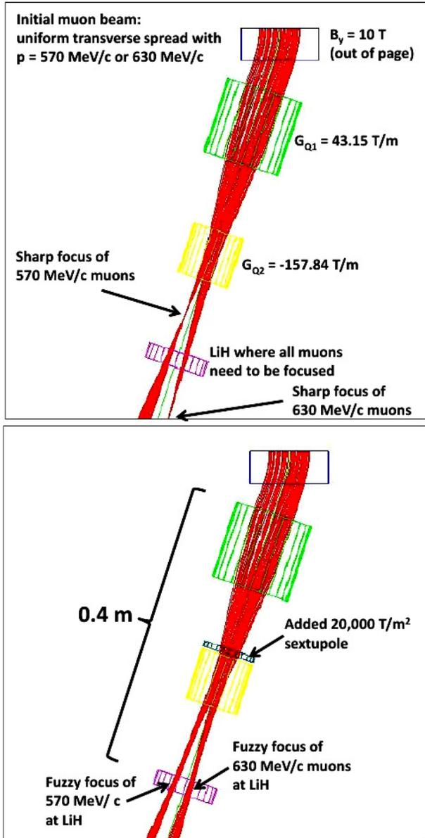
Figure 5: Half Cell with a bending magnet and sextupole to test chromaticity correction.
