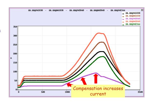
Measured Quadrupole currents along the machine cycle with compensation of gradients in bends during ramp
