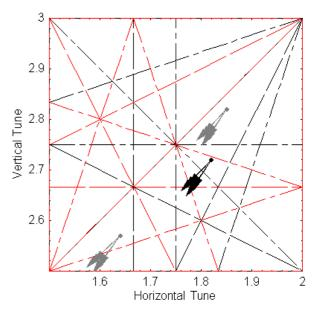
■ Lattice functions for one half of LEIR and working point (black: nominal working point, grey: alternative working points)
