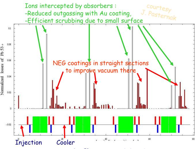
Loss pattern of Pb<sup>53+</sup> ions around the LEIR ring with collimators and homogeneous gas density
