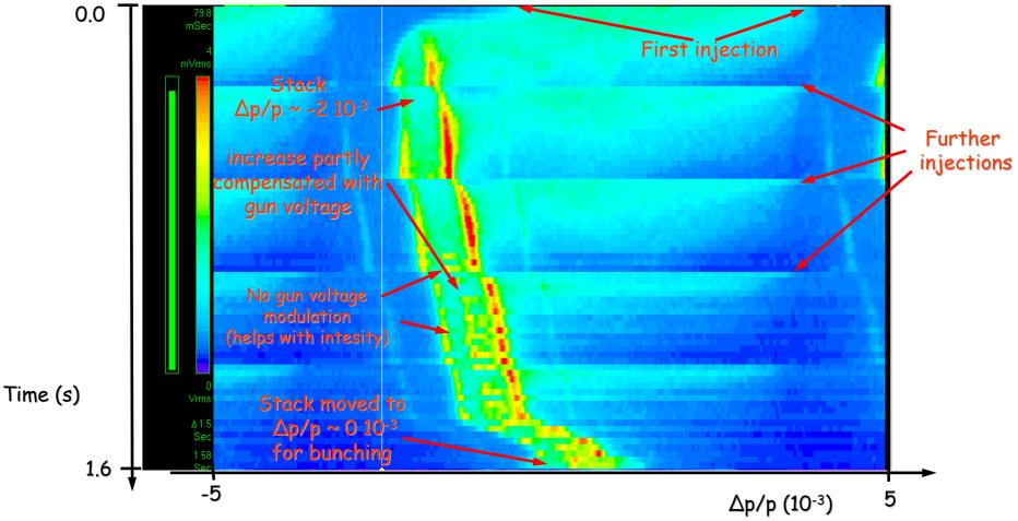
■ Evolution of longitudinal Schottky spectra during accumulation (measured with a commercial FFT spectrum analyser)
