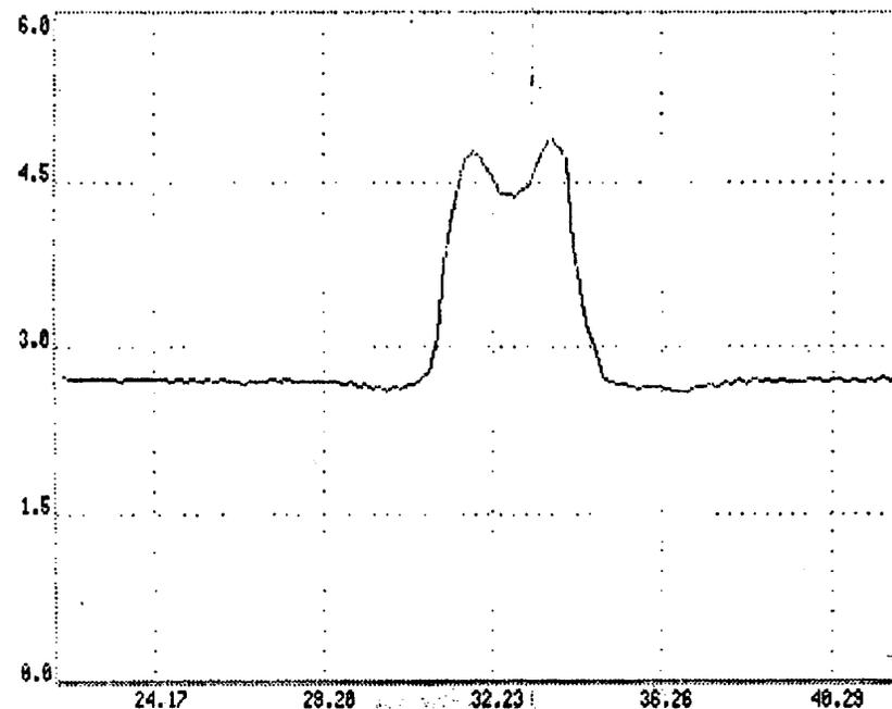
Figure 1: A double peak horizontal beam profile for 250 MeV/u  $O^{8+}$ . The scale on the  $x$ -axis is in mm.
