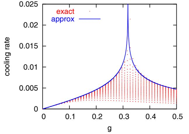
Figure 4: Comparison of actual values of  $Re(\lambda)$  versus gain with those obtained from equation (12) with  $X = 0$  for a rectangular frequency distribution with  $N = 51$ . The numerical solution had one eigenmode with a monotonically growing eigenvalue, which is not fully shown.
