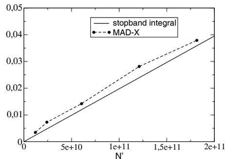
Figure 7: Full rms beam width after 1000 revolutions calculated using MAD-X compared to the half integer stopband integral  $J_7$  from equation 10.
