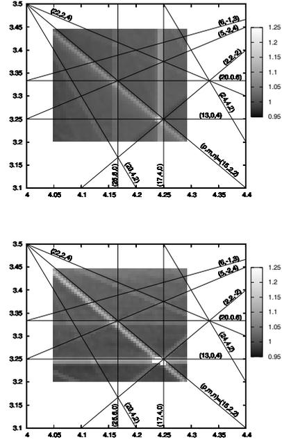
Figure 2: Relative rms beam width in  $x$  and  $y$  direction, upper and lower picture, respectively. The colour scale is within  $w_{\text{rel}} \leq 1$  (dark grey) and  $w_{\text{rel}} \geq 2$  (white).
