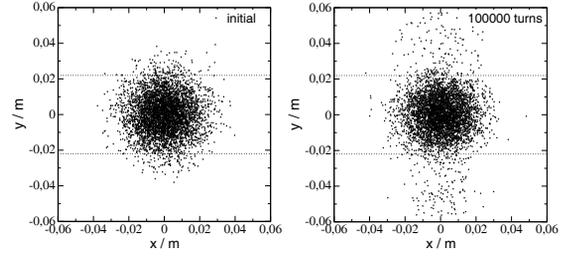
Figure 4: Spatial beam profile for  $\sigma_{i,x} = \sigma_{i,y} = 0.5b$  at the beginning of a run and after 100000 revolutions. The working point is  $\nu_x = 4.1$ ,  $\nu_y = 3.245$ .
