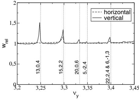
Figure 3: Relative beam width as a function of the vertical tune within the range  $\nu_y \in [3.1, 3.45]$  for one horizontal tune  $\nu_x = 4.2$ . So, this figure is an extract of figure 2.
