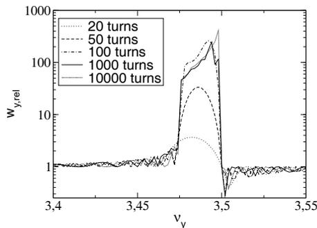
Figure 6: Relative vertical rms beam width  $w_{y,rel}$  after different numbers of revolutions. Note, that it is  $\sigma_{i,y} = 0.01 b$  and, so  $w_{y,rel} = 100$  refers to an absolute final rms beam width  $\sigma_{f,y} = b$ . It is  $\nu_x = 4.2$ .
