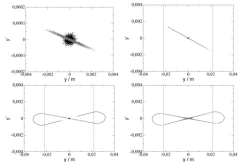
Figure 5: Vertical phase space plot for an initial beam width  $\sigma_{i,y} = 0.01 b \ll b$  at  $\nu_x = 4.2$ ,  $\nu_y = 3.45$  after several number of revolutions:  $N_{rev} = 20, 50, 100, 10000$ . The vertical straight lines in pictures 2 – 4 denote the radius of the electron beam  $b$ . The black points in the centre denote the initial positions of the particles in phase space.
