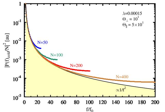
Figure 7: Particle number dependence of cold integrated Schottky signals (divided by  $N^2$ ) vs. harmonic.
