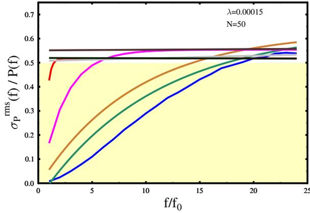
Figure 4: Rms width over average value of the integrated Schottky spectra of Fig. 3a for various temperatures (same color code).
