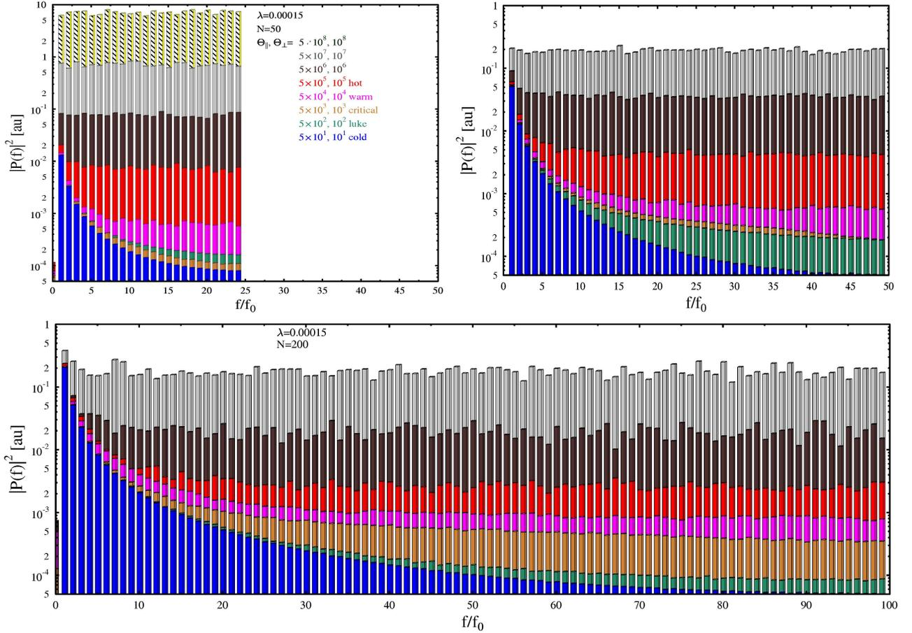
Figure 3: Calculated integrated Schottky spectra for the linear density  $\lambda = 0.00015$  at various longitudinal and transverse temperatures and various number of particles  $N=50$  (a: top left),  $N=100$  (b: top right) and  $N=200$  (c: bottom).
