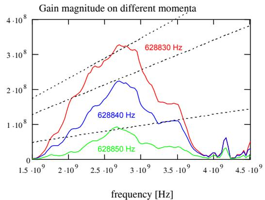
Figure 10: Stacktail gain before installation of an equalizer.
