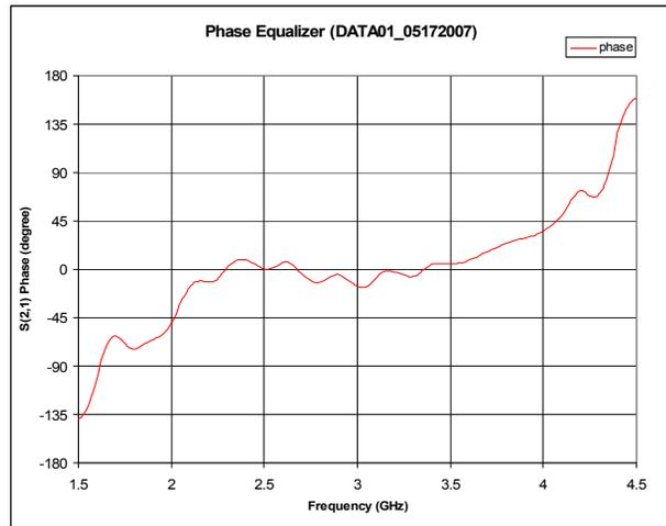
Figure 3: Phase of a phase equalizer part.
