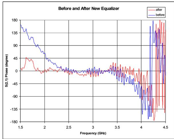
Figure 8: Phase of transfer function before and after installation of an equalizer.
