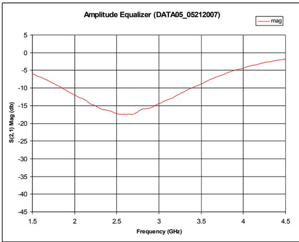
Figure 6: Amplitude of an amplitude equalizer part.
