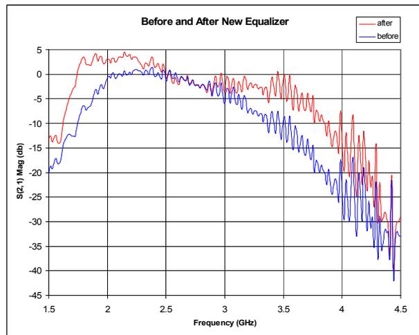
Figure 9: Amplitude of transfer function before and after installation of an equalizer.
