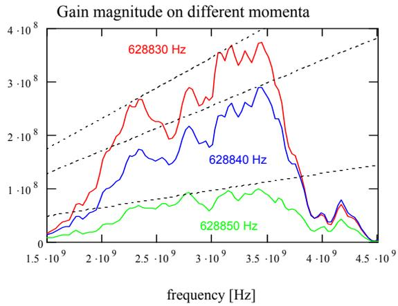
Figure 11: Stacktail gain after installation of an equalizer.
