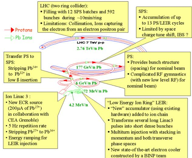
Figure 1: Overview of the LHC ion injector chain.
