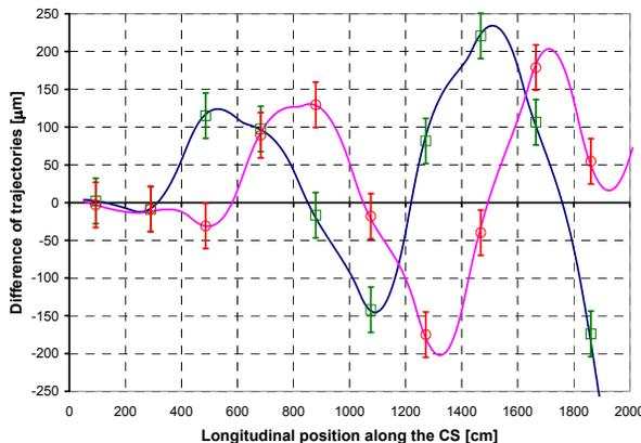
Figure 1: Difference of trajectories taken 3 months apart. Green squares: Horizontal; Red circles: Vertical.  $I_b = 100$  mA, on-axis. The solid lines are fitted trajectories using the measured magnetic fields and solenoid-to-solenoid magnetic offsets as fitting parameters.
