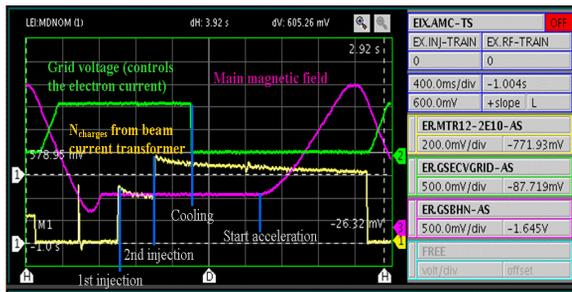
Figure 1: A standard 3.6s LEIR cycle during which 2 LINAC pulses are cooled-stacked in 800ms at an energy of 4.2 MeV/n. After bunching the Pb ions are accelerated to 72 MeV/n for extraction and transfer to the PS.
