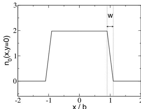
Figure 1: Normalised charge density profile used for the electron beam as provided by the beambeam element of MAD-X [3] as a function of  $x$  for  $y = 0$ . An edge layer with a width  $w = 0.01 b$  was used in the calculations.
