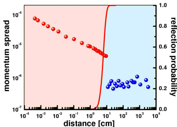
Figure 2: Momentum spreads of an  $U^{92+}$  beam at 360 MeV/u. The red line is the calculated reflection probability, see below. After Steck [3] and Hasse [4].
