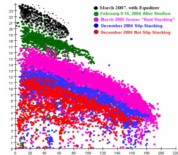
Figure 2: Dependence of antiproton production rate (units of  $10^{10}$  hour<sup>-1</sup>) on stack size (units of  $10^{10}$ ) during Run II.
