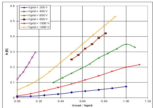
Figure 2: Electron beam current as a function of  $V_{cont}/V_{grid}$  for  $E_e = 2.3$  keV.
