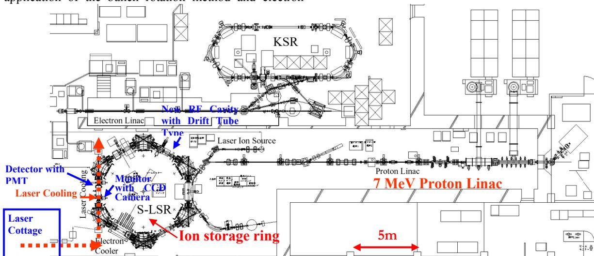
Figure 1: Layout of the radiation controlled experimental room where S-LSR is installed. As the injection beam for S-LSR, 7 MeV proton from the linac and 40 keV  ${}^{24}\text{Mg}^+$  ion beam has been utilized up to now.
