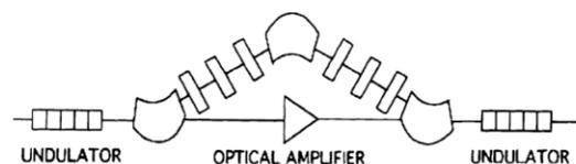
Figure 1: Schematic of an optical stochastic cooling insertion in a storage ring.
