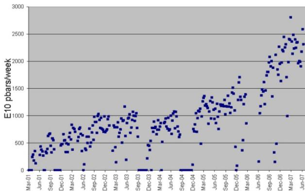
Figure 1: Weekly antiproton production rate during Run II (2001-2007).
