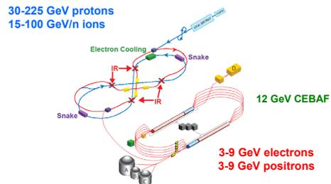
Figure 1: A schematic drawing of ELIC ring-ring design.
