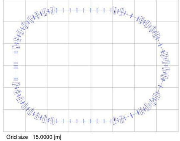
Figure 1: Main magnet layout of the cooler ring.
