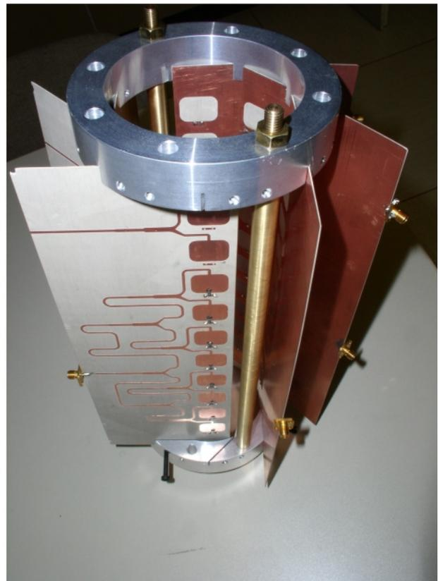
Figure 1: Octagonal pickup structure, equipped with 6  $\lambda/4$ -electrode rows.
