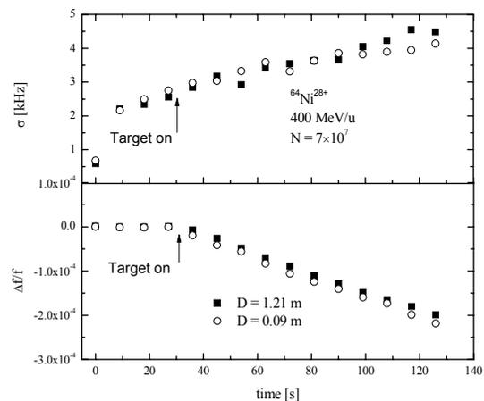
Figure 1: Relative change of the mean frequency  $\Delta f/f$  caused by the energy loss due to the internal target (Kr-target  $6 \times 10^{12}$  atoms/cm<sup>2</sup>). The change of the width of distribution  $\sigma$  with the time.
