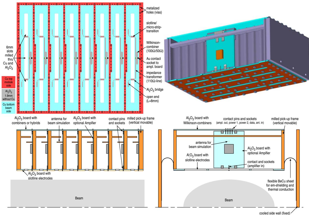
Figure 1: Layout of eight slot pick-up module prototype on a scale of 1:3.
