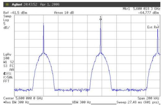
Figure 1: A Schottky spectrum showing coherent components.
