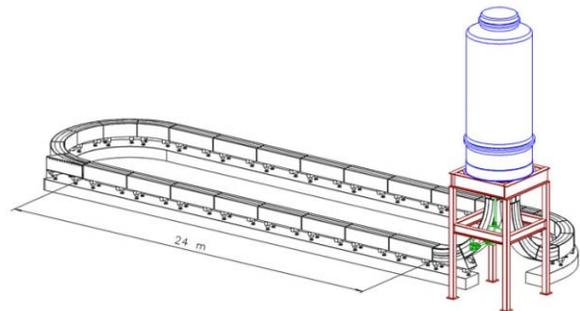
Figure 1: Layout of the HESR electron cooler showing the Pelletron tank and the beam line system of solenoid magnets. The length of the interaction section is 24 m.
