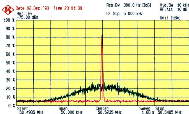
Figure 1: Early (1993) Schottky spectra from the ESR before (green) and after (red with  $\delta p/p = 2 \times 10^{-5}$ ) electron cooling.
