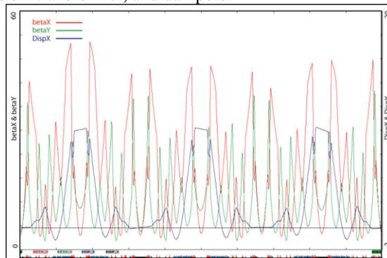
Figure 1: Accumulator Twiss-functions. Red and green traces show the horizontal and vertical beta-functions. The horizontal dispersion is shown with the blue trace.
