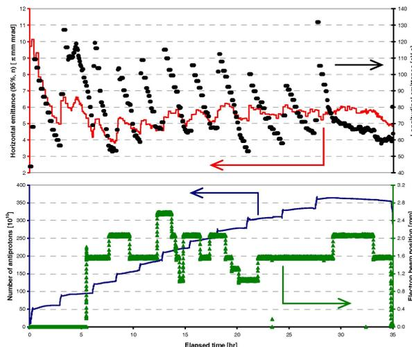
Figure 1: Example of the cooling sequence and electron beam utilization during a storage cycle. Bottom plot - Solid blue: Number of antiprotons; Green triangles: Electron beam position; Top plot - Solid red: Transverse (horizontal) emittance measured by the 1.75 GHz Schottky detector; Black circles: Longitudinal emittance measured by the 1.75 GHz Schottky detector. The electron beam current is kept constant (100 mA).
