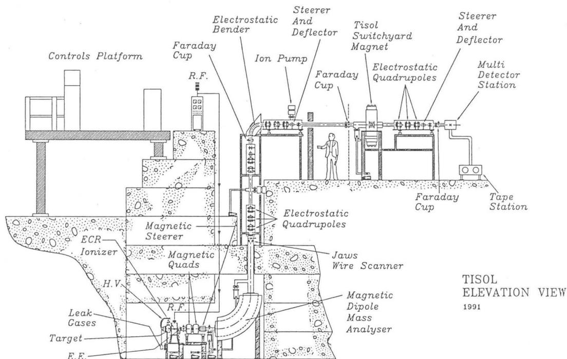
Fig. 1. Elevation view of TISOL.
