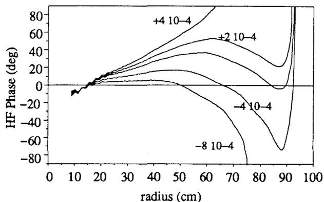
Figure 1 : Phase histories for a given particle in the reference field and fields with  $\Delta B/B = +2, +4, -4$  and  $-8 \cdot 10^{-4}$ .
