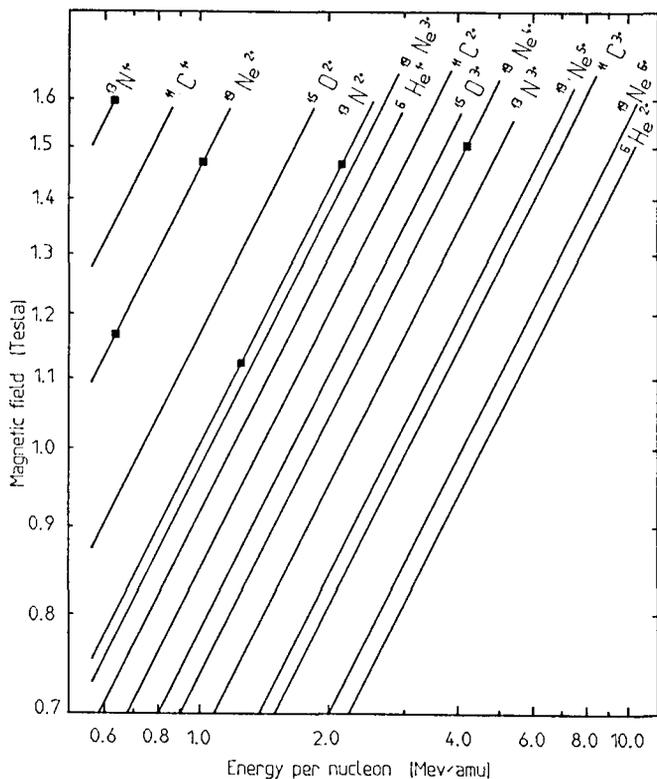
Figure 3 : Operating diagramme for RIB acceleration with CYCLONE.
