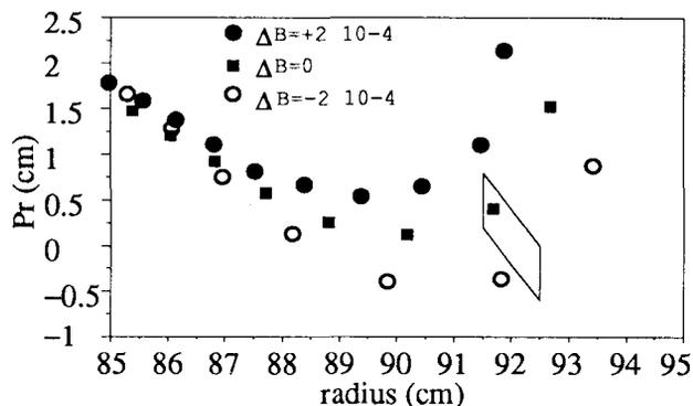
Figure 2 : Acceptance of the extraction system and trajectories of a particle in the reference field and fields with  $\Delta B/B = +2$  and  $-2 \cdot 10^{-4}$ .
