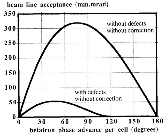
Fig. 3. Acceptance of a 200 m long beam handling made of FODO cells with or without defects on quadrupole positions (see text). Our channel having 400 m we will have to recenter the beam along the path.
