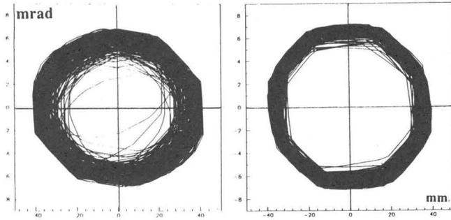
Fig. 4. Acceptances of a FODO 200m long line for 200 sets of mispositionings (see text for conditions).before and after recentring of the beam after each 50m, taking into account of the 1 mm RMS error of monitor positioning.
