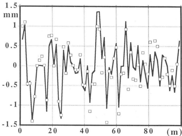
Fig. 5. Example of a simulation of a set of misalignments of quadrupoles over 100 m : real values (arbitrary linked by a solid line) and estimated values (square points) (see text for conditions)
