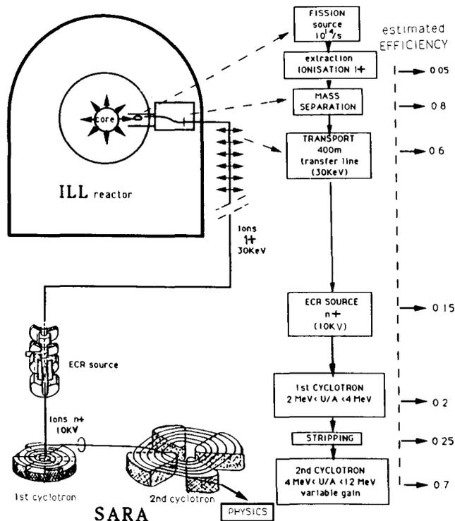
Fig.1. Schematic diagram of the projected production, ionization, acceleration of exotic beams facility P.I.A.F.E. at Grenoble
