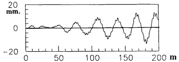
Fig. 2. The central trajectory is plotted along a 200 m FODO structure and for one set of mispositionnings (see text).
