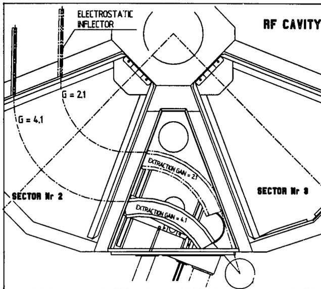
Fig. 6. The proposed extraction system allows the second cyclotron having a continuously varying gain between 2.1 and 4.1.
