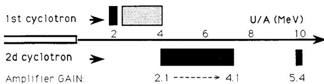
Fig. 7. Energies for Xenon. 4 MeV/amu is directly obtained with the first cyclotron. Presently energy gain G of the second cyclotron is  $G = 5.4$ , allowing only 10.5 MeV/amu. It is expected a variable extraction :  $2.1 < G < 4.1$  allowing to cover the energy range of 4 to 7.8 MeV/amu (and 10.5). Because stripping effect is not large enough, only 1.9 MeV/amu from the first cyclotron can be injected in the second one.
