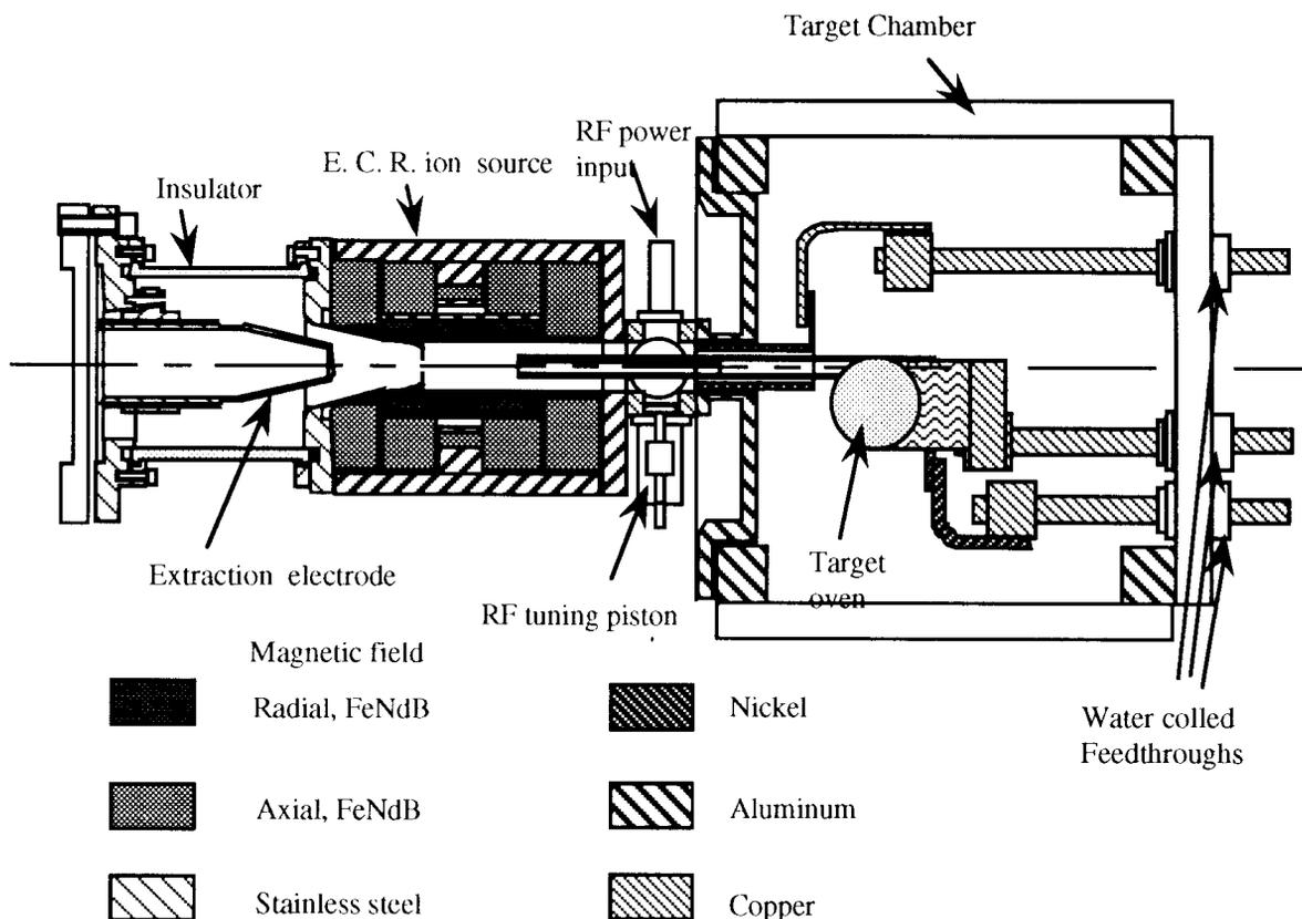
Fig 2 Schematic view of the target and ECR ion source.
