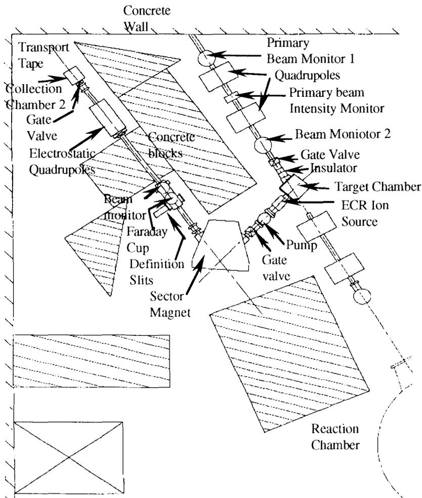
Fig.1 Schematic top view of the separator test bench installed in the experimental room D2 at GANIL.
