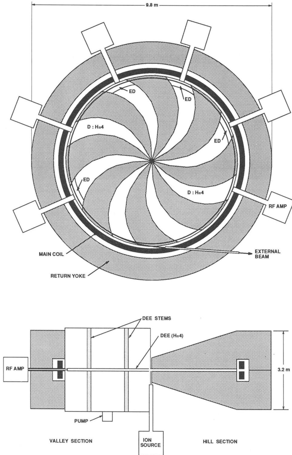
Fig. 3. 600 MeV proton cyclotron, plan and elevation views.
