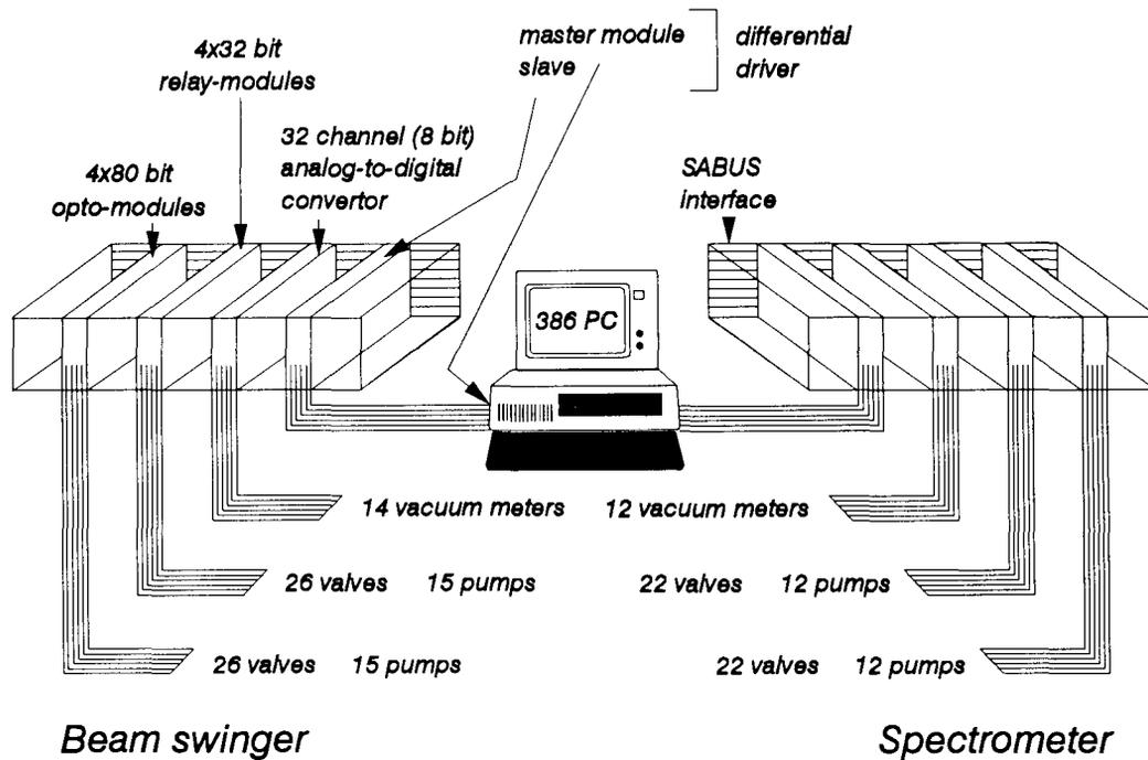
Fig. 1. A schematic view of the instrumental node for the two vacuum systems.
