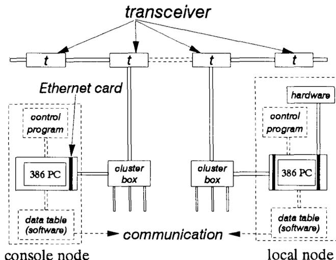
Fig. 4. A schematic representation of the Ethernet network.
