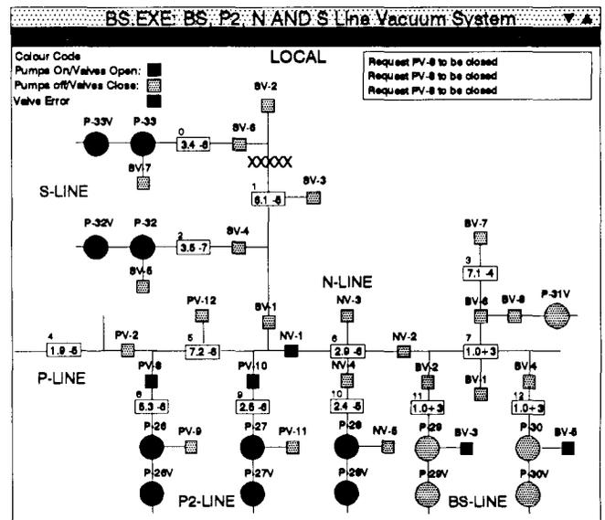
Fig. 2. A screen copy of the colour monitor video display of the 'beam swinger' vacuum system.
