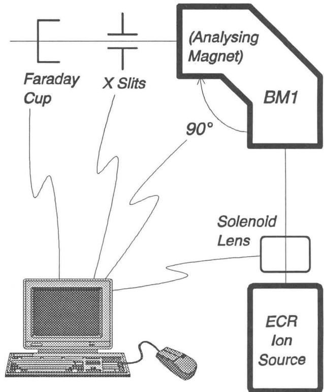
Fig. 2. Schematic Layout of the ECR Ion Source.
