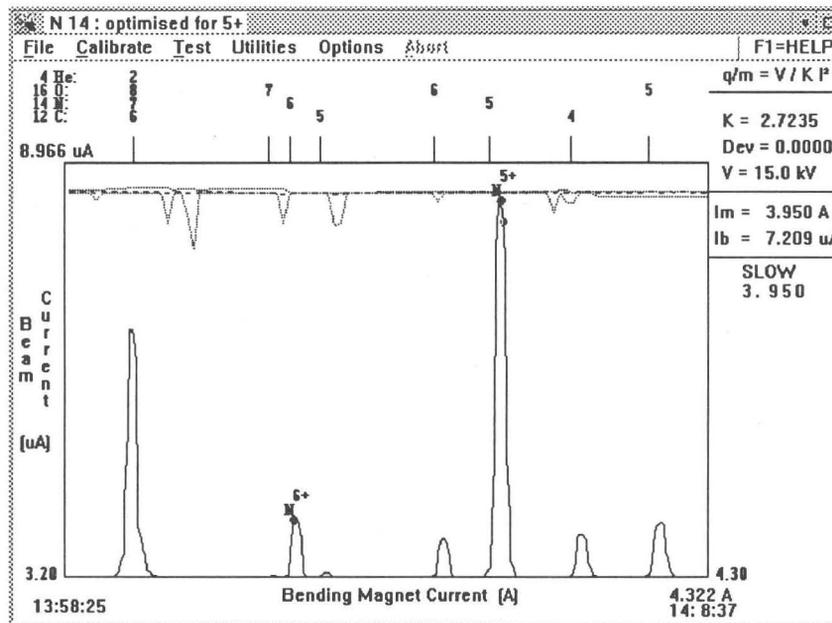
Figure 3. ECR ion source plot for a  $^{14}\text{N}^{5+}$  beam.
