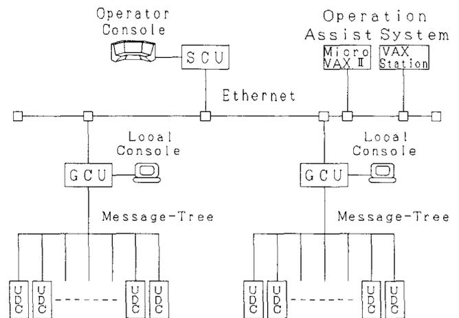
Fig. 1. Architecture of the JAERI AVF cyclotron control system
