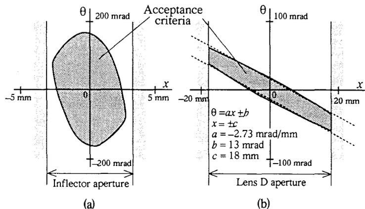
Fig. 3. Acceptance criteria of the axial injection block. (a) For inflector (b) following lens D.
