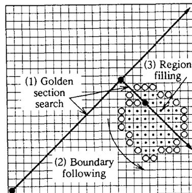
Fig. 4. Process used by the "search method" to obtain an FSR.
