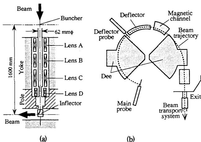
Fig. 2. Schematic of the axial injection block (a) and the extraction region (b).
