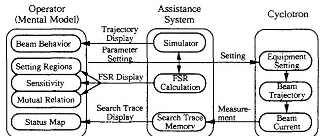
Fig. 6. Block diagram of information flow in the operator assistance system.
