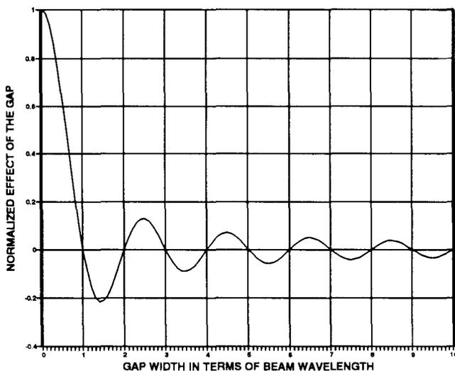
Fig. 3. Normalized gap effectiveness as a function of gap width.
