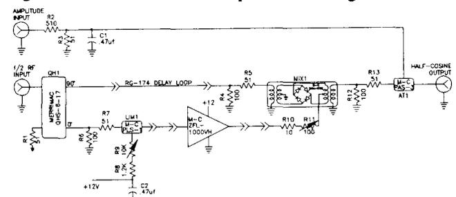
Fig. 8. Schematic diagram of half-cosine wave generator.
