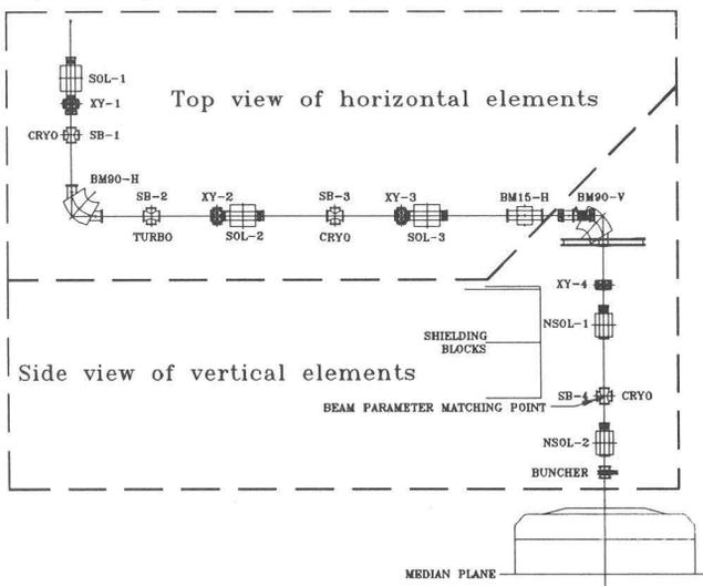
Fig. 1. Schematic of the axial injection system for the K500 cyclotron.
