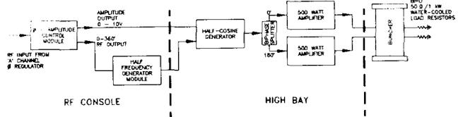
Fig. 7. Block diagram of buncher electronics system.
