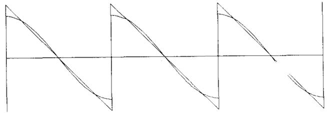
Fig. 4. Idealized sawtooth and half-cosine wave forms.
