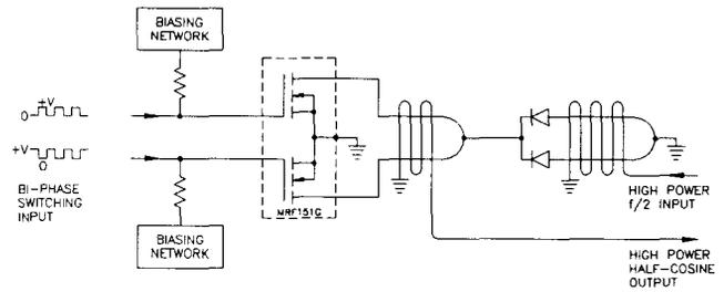
Fig. 9. Preliminary circuit design for a high power half-cosine generator.
