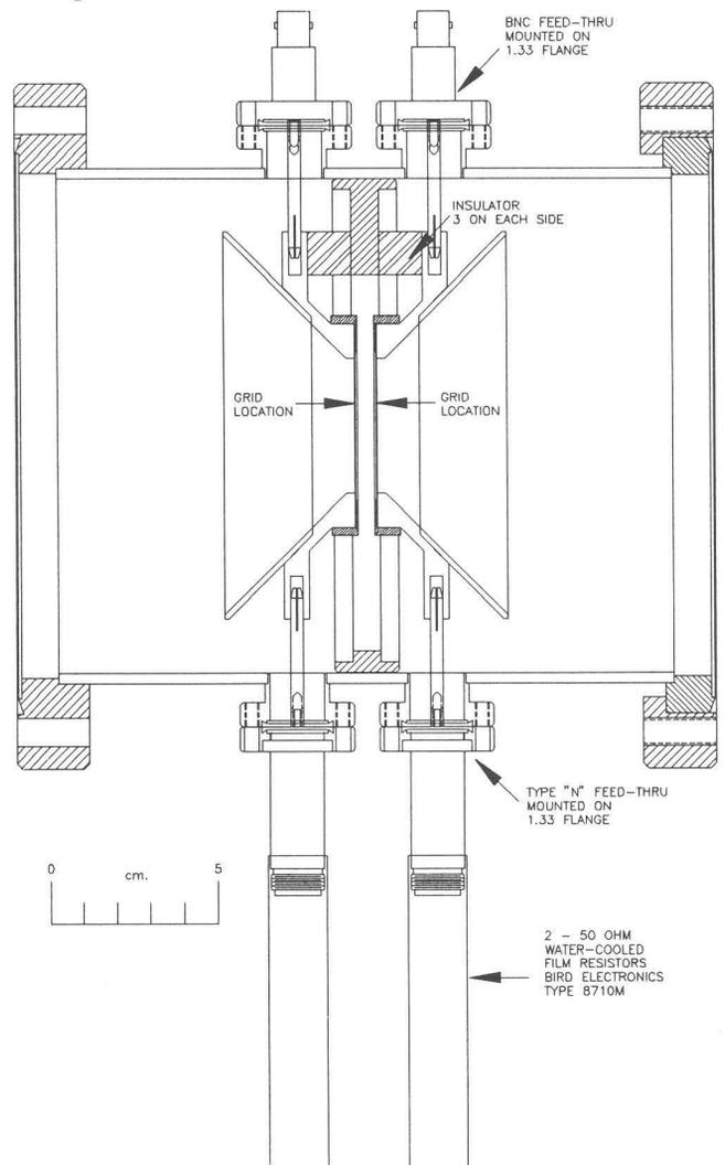
Fig. 2. Sectional view of the single gap buncher.
