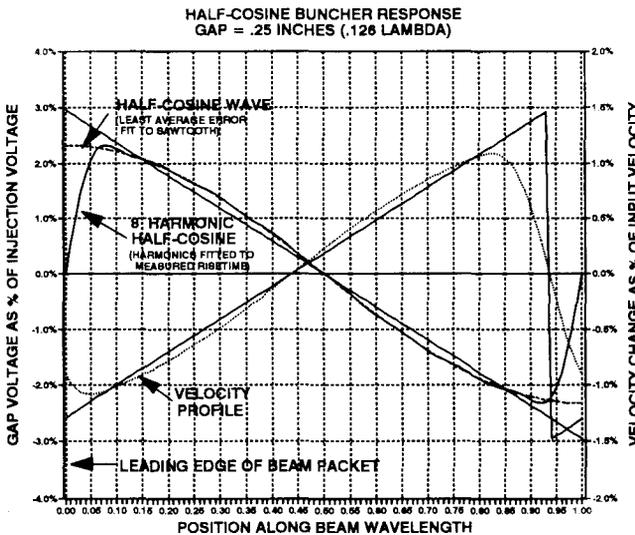
Fig. 6. Half-cosine voltage wave form and particle velocity profiles reconstructed from Fourier components. Velocity profile is constructed from gap effect modified components.
