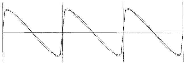
Fig. 5. Sawtooth and half-cosine wave forms with 10% risetimes.
