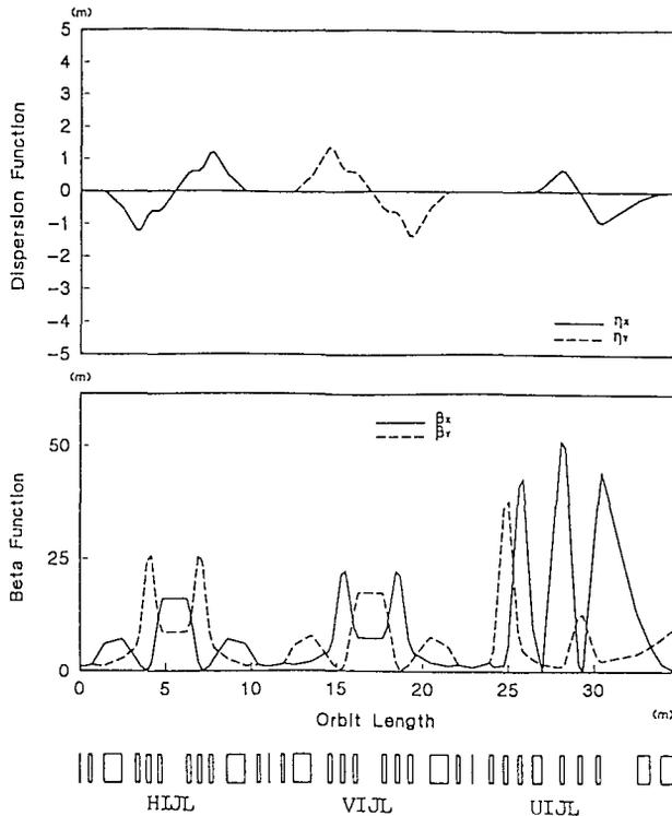
Fig. 2. Beta and dispersion functions in the IN-JBT to the upper ring.
