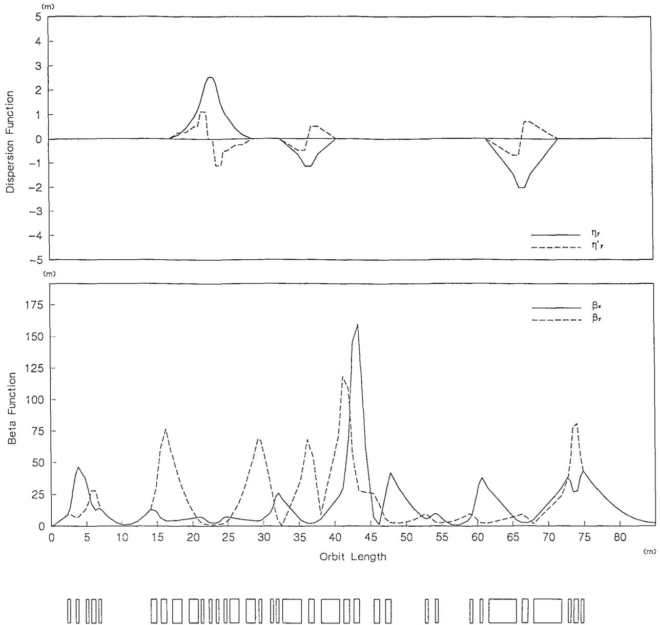
Fig. 4. Beta and dispersion function of the vertical beam line to the isocenter of the treatment room A.
