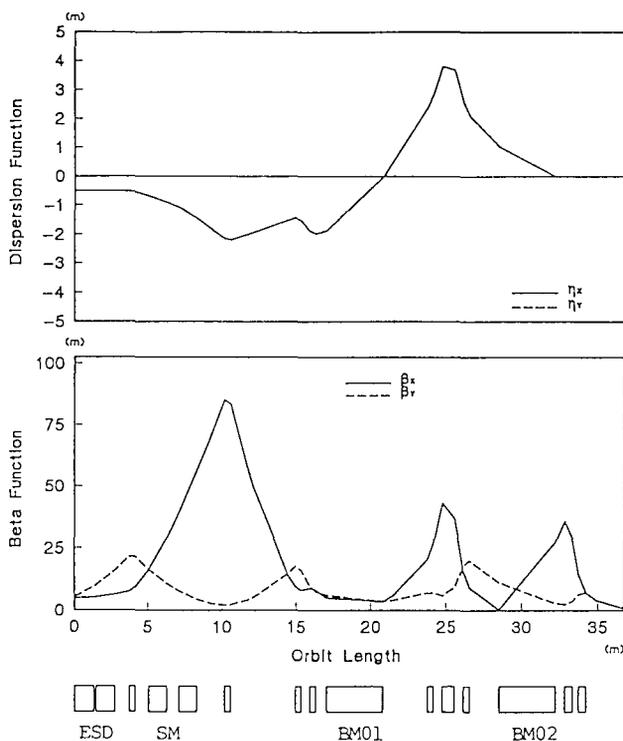
Fig. 3. Beta and dispersion functions in the EXBT.
