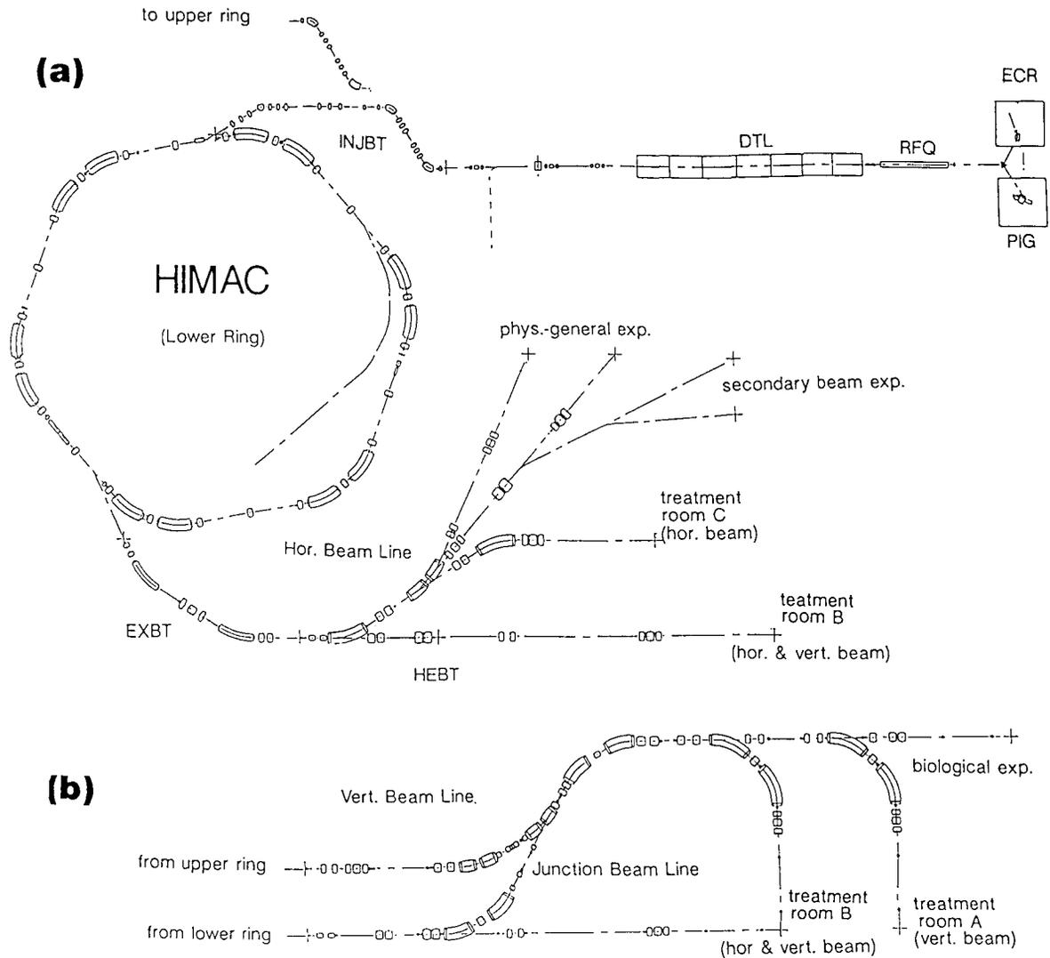
Fig. 1. (a) A plane view of the HIMAC. (b) A side view of the vertical beam line in the HEFT.
