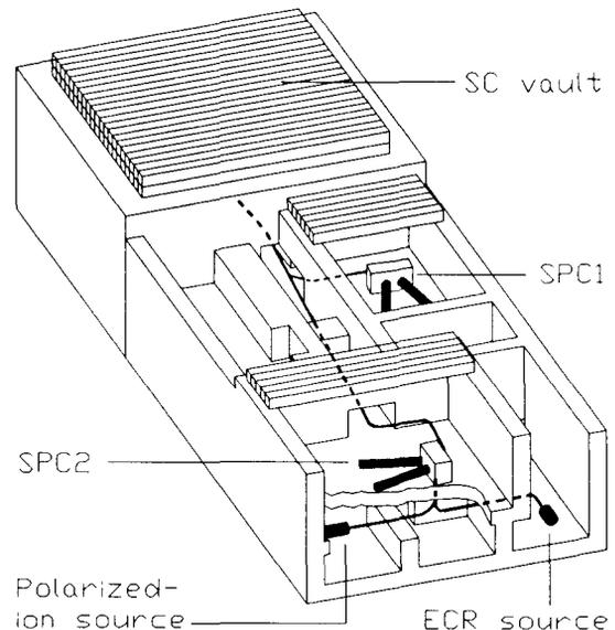
Fig. 1. Layout of the transfer beamlines at NAC.
