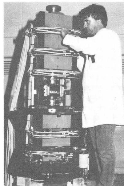
Fig. 4. Rotatable 2-triplet quadrupole telescope, prior to mounting in the axial injection beamline below SPC2.
