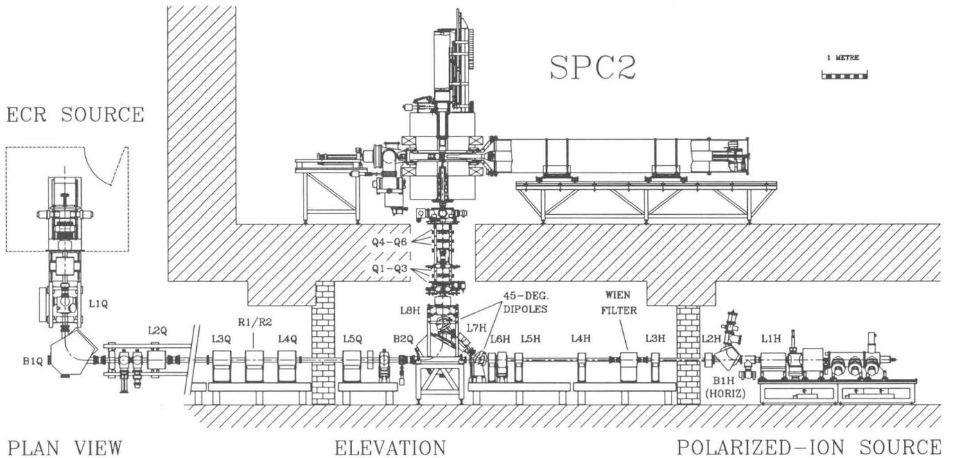
Fig. 2. The transfer beamlines between the ECR and polarized-ion sources and the injector cyclotron SPC2.
