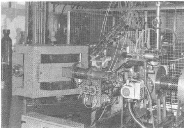
Fig. 3. The first 90° dipole of the "twisted achromat" in the beamline from the ECR source which is visible in the background.
