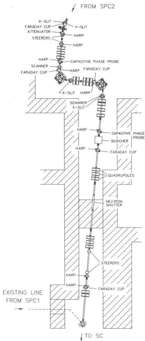
Fig. 6. The transfer beamline between SPC2 and the sector cyclotron, which joins the existing transfer beamline from SPC1.
