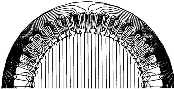
Fig. 5. POISSON plot of the field lines calculated for a sinusoidally wound  $x$ - $y$  steering magnet, shown here operating in the  $x$ -direction only.
