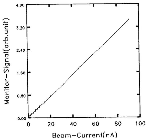
Fig.3. Signal from the inductive beam-current monitor, measured as function of beam intensity, simulated by a chopped current.
