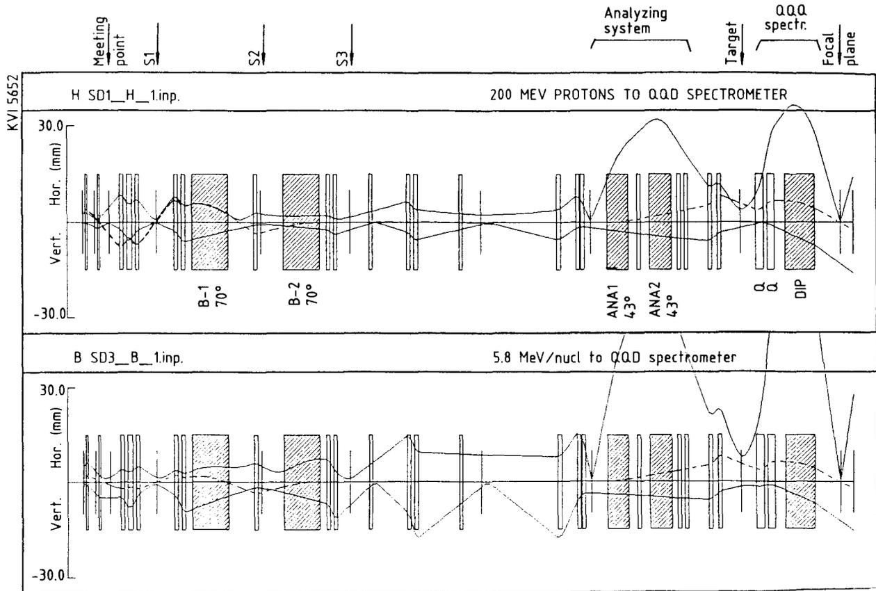
Fig. 2. Envelopes and dispersion lines (dashed) for two AGOR beams in high-resolution mode to the QDD magnetic spectrometer.
