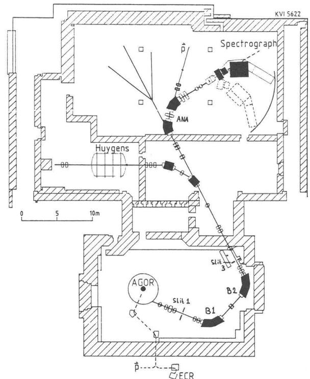
Fig.1. AGOR experimental area and beam-line layout at the KVI.
