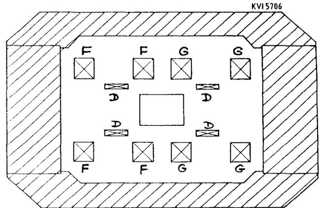
Fig.2. Cross-section of shielding tube and first focussing element. F and G are gradient coils, D is the dipole coil.
