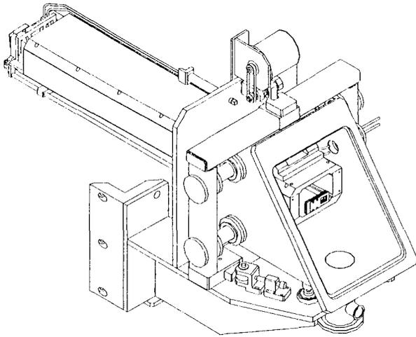
Fig.3. Perspective view of the channel with its support structure. The buffer volume for liquid helium is not shown.
