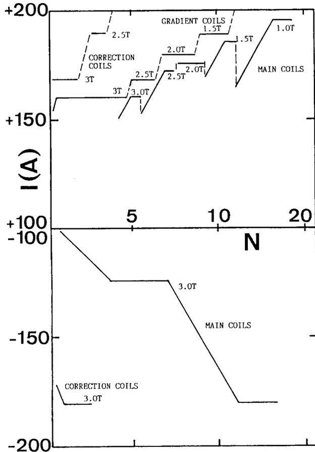
Figure 5: Results of the quench test done on EMC2-2
