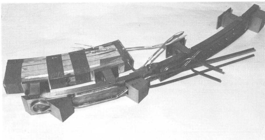
Figure 4: EMC2-1 connected to the 80K shield. The hinge construction between EMC2-1 and EMC2-2 is visible
