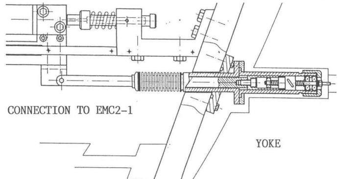
Figure 3: The mechanical construction of a guide/slide mechanism
