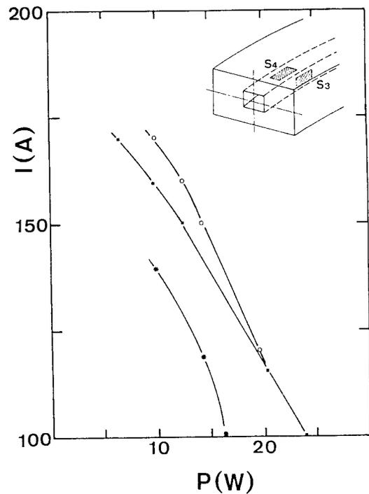
Figure 6: Quench current of EMC2-2 in relation to a simulated beam load on the bore of the element
