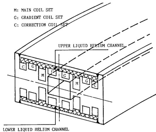
Figure 1: The geometry of the EMC2 coil system
