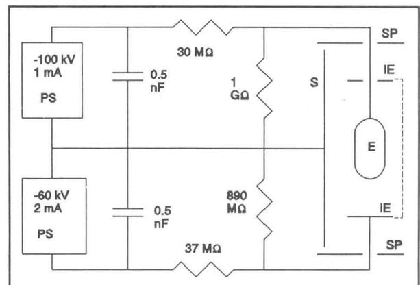
Fig. 4 Schematic of the system to supply high voltage to the model deflector electrode and the intermediate electrodes.
