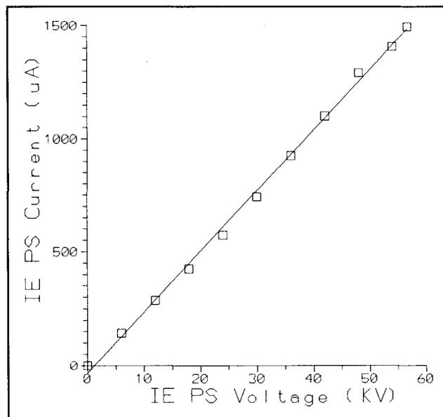
Fig. 6 Feed insulator characteristic for the intermediate electrodes.
