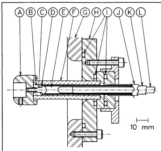
Fig. 5 Schematic of the high-voltage feed insulator for the intermediate electrodes.
