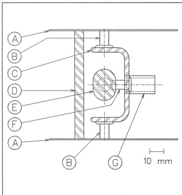
Fig. 2 Cross section of the model intermediate electrode. A - sparking plates; B - insulator; C - intermediate electrode; D - septum; E - deflector electrode; F - insulator; G - metal post.
