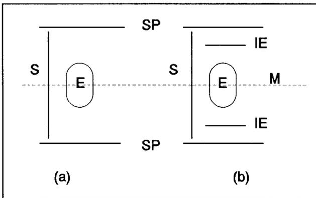
Fig. 1 Schematic of the deflector electrodes, (a) traditional arrangement, and (b) with intermediate electrodes (IE). E - deflector electrode; M - cyclotron midplane; S - septum; SP - sparking plates.
