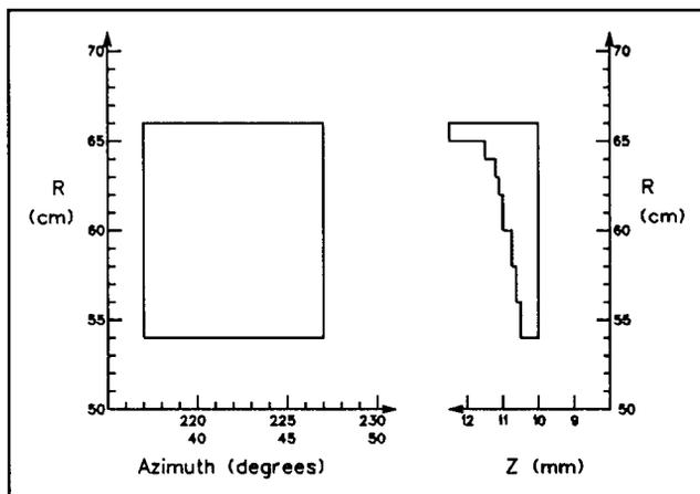
Fig. 4 Schematic of the iron used to compensate average field perturbations caused by the hill lens modifications.
