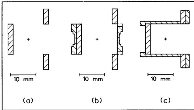
Fig. 2 Cross section of hill lenses: (a) lens 1 without modifications; (b) modified lens 1; (c) modified lens 2.
