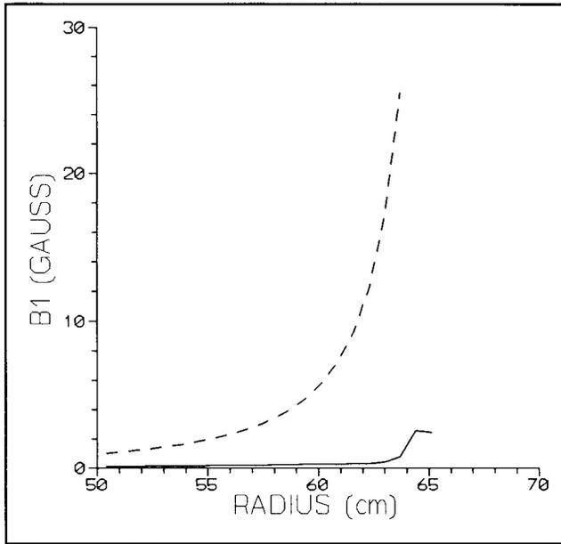
Fig. 3 Plot of first harmonic perturbation fields B1 from the iron additions to the hill lenses; dashed line, uncompensated; solid line, compensated.
