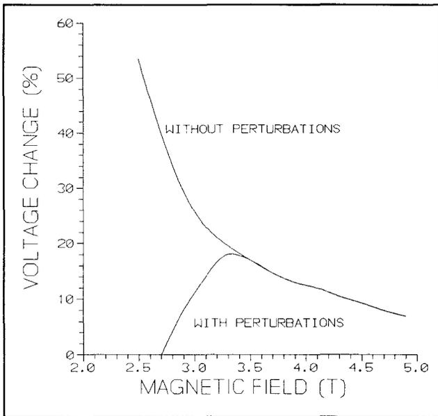
**Fig. 6** Plot of the deflector voltage change resulting from enhanced magnetic deflection in the hill lenses.
