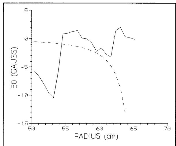
Fig. 5 Plot of the average field perturbations generated by the hill lens modifications; dashed line, uncompensated; solid line, compensated.
