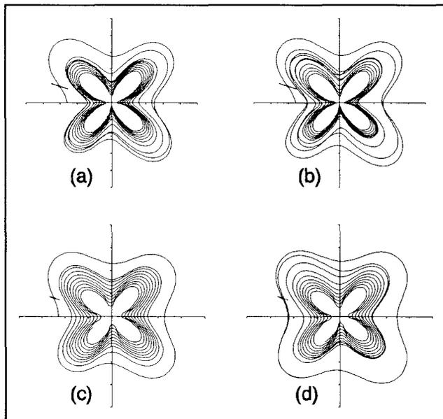
**Fig. 7** Orbit plots for C, 45 MeV/u without (a) and with (b) lens modifications; and for Cl, 8.5 MeV/u without (c) and with (d) lens modifications. Scale interval: (a) and (b), 1 cm; (c) and (d), 2 cm.
