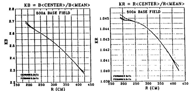
Fig. 7. Comparison of  $K_b$  and  $K_r$  values among the six sectors at 500A excitation.
