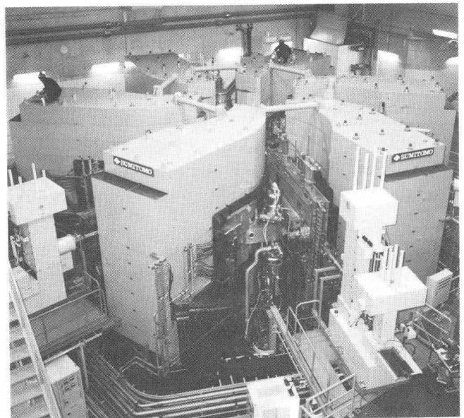
Fig. 2. Photograph of sector magnets installed in the cyclotron vault.
