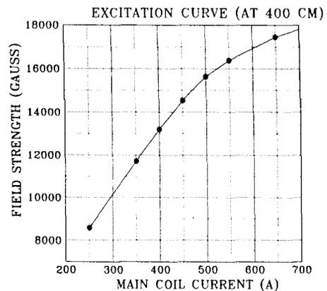
Fig. 4. Excitation characteristic of a sector magnet.
