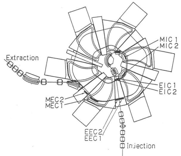
Fig. 1. Schematic mid plane view of the magnet system of the ring cyclotron.
