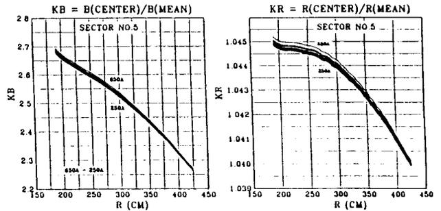
Fig. 6.  $K_b$  and  $K_r$  values of the No.5-sector at the seven main coil levels.
