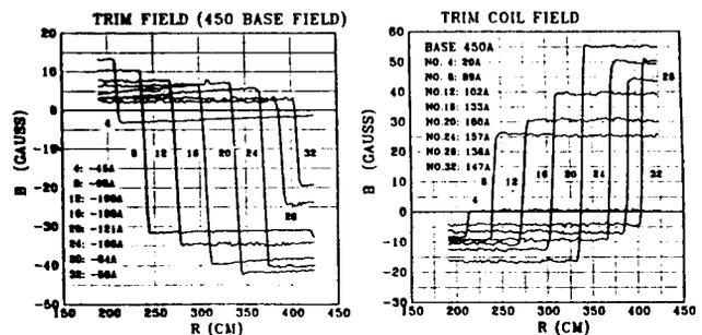
Fig. 8. Examples of the trim coil field distributions along the sector center line at the field gradients corresponding to the 400 MeV protons and 400 MeV alpha particles at 450A base field.
