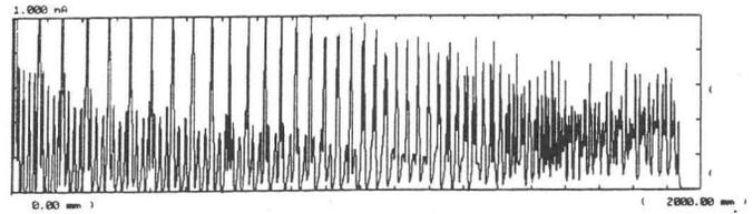
Fig. 9. Beam current measured by a wire probe from injection radius to extraction radius.
