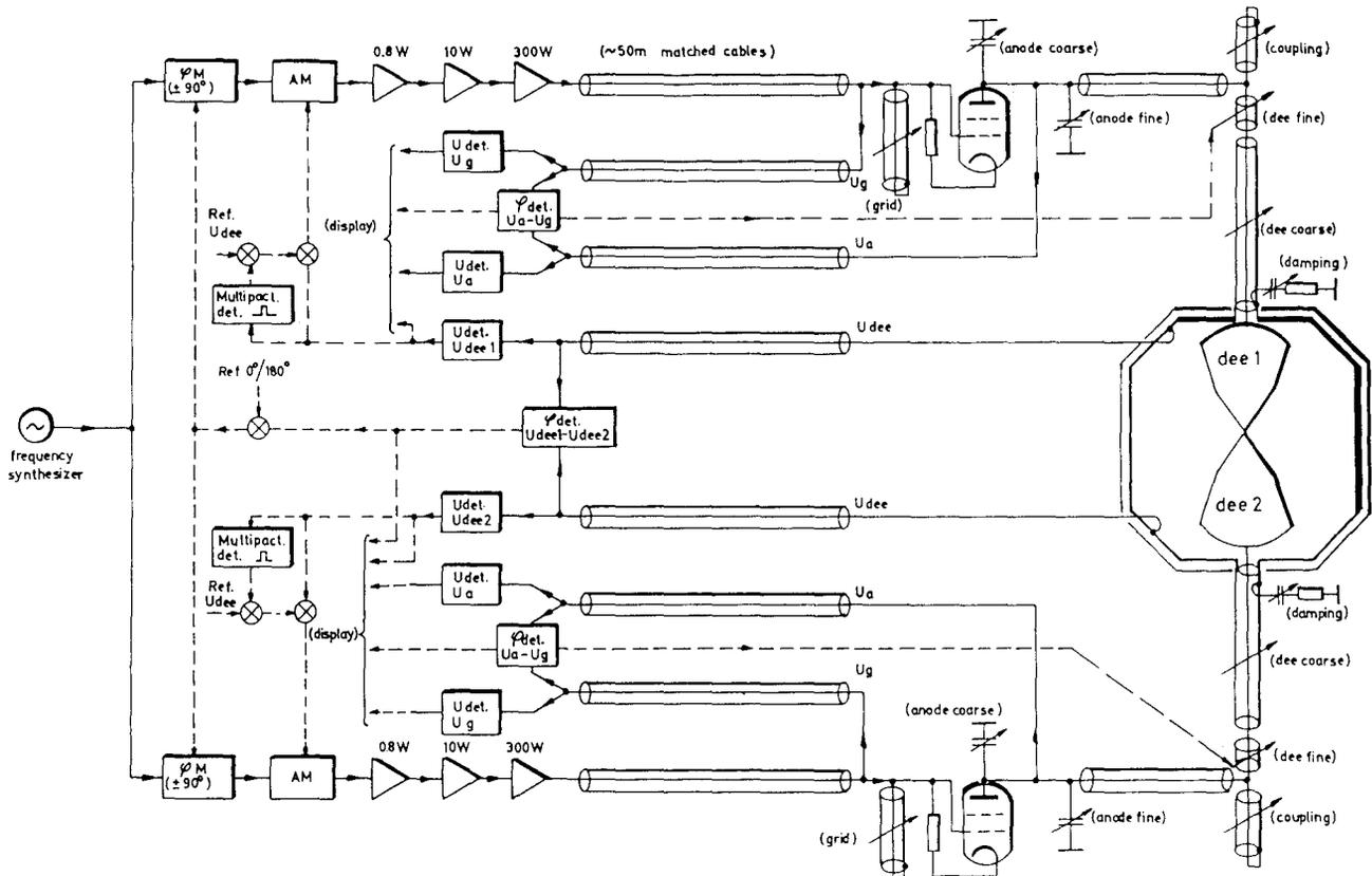
Figure 3. Block diagram of the RF system (CW mode)
