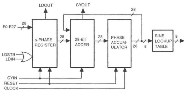
Figure 6. Numerically controlled oscillator (FM source).
