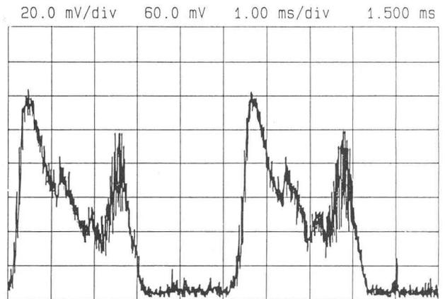
Fig. 9. Faraday cup measurement of a stretched 180 MeV proton beam with approx. 50 % duty cycle.
