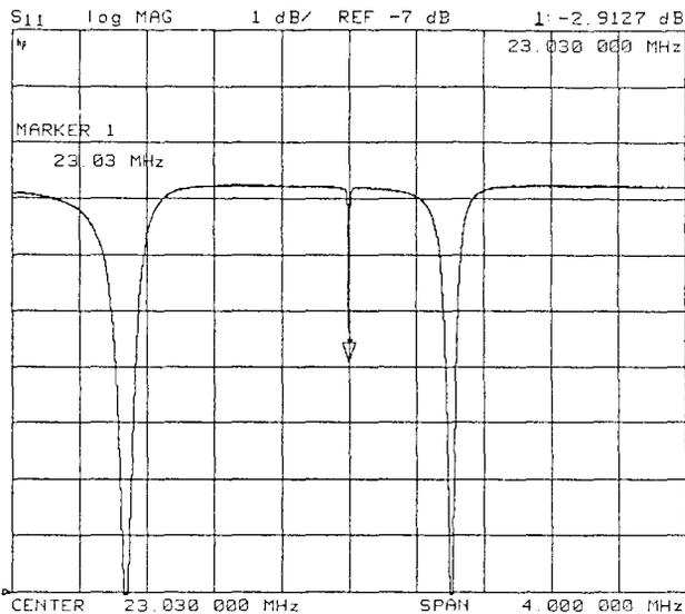
Figure 3. Cavity & transmission line modes.
