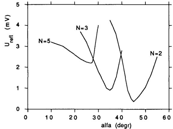
Fig. 14. Reflected wave vs angle of loops.
