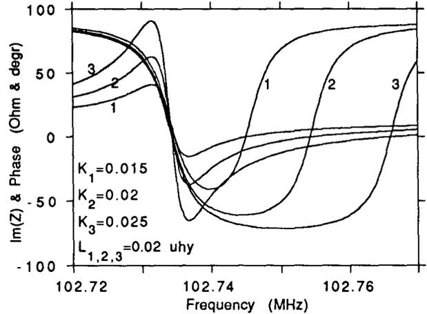
Fig. 2b. Reactance & Phase of coupling loop.
