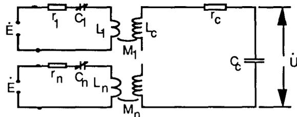
Fig.10. Simplified diagram of multi-loop cavity excitation.
