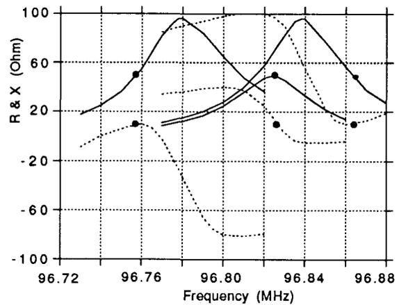
Fig. 7. Active & reactive resistances of coupling loop matched with cavity.
