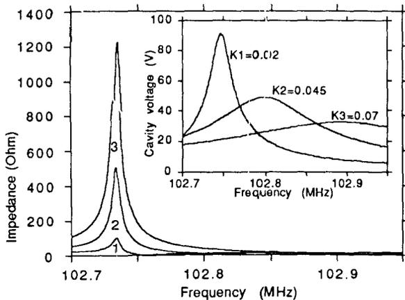
Fig. 2a. Coupling loop resonance characteristics.
