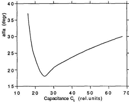
Fig. 8. Angle of loop vs compensating capacity.
