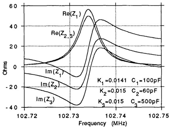
Fig. 9. Capacitance variation at the same coupling factor.
