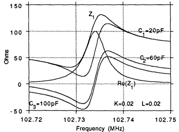
Fig. 3. Compensation of coupling system inductance.
