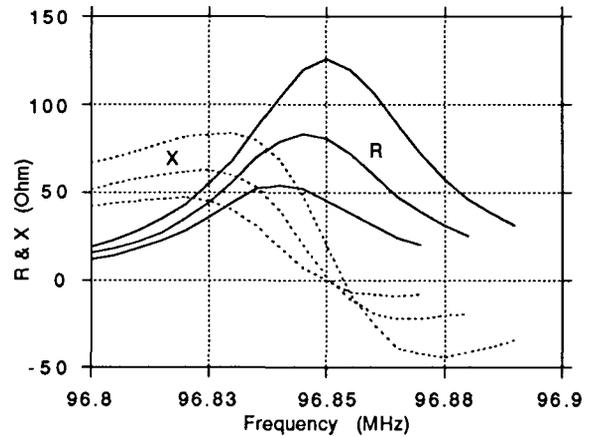
Fig. 6. Active & reactive resistances of coupling loop.
