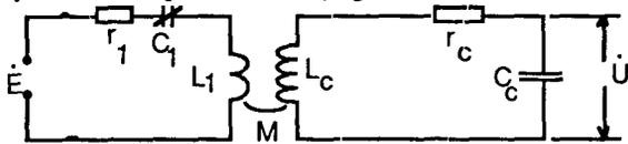
Fig. 1. RF system as the coupled circuit system.
