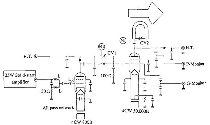
Fig. 7. Schematic diagram of the amplifier system.
