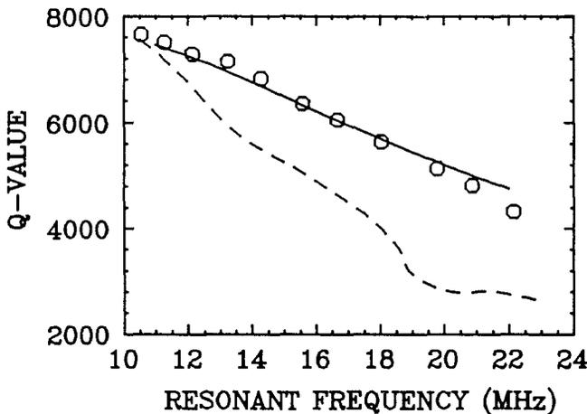
Fig. 5. Frequency dependence of Q-value. The solid line shows 75 % of the calculated value based on one-dimensional transmission line approximation. The dashed line shows the measured value of the movable panel type cavity.
