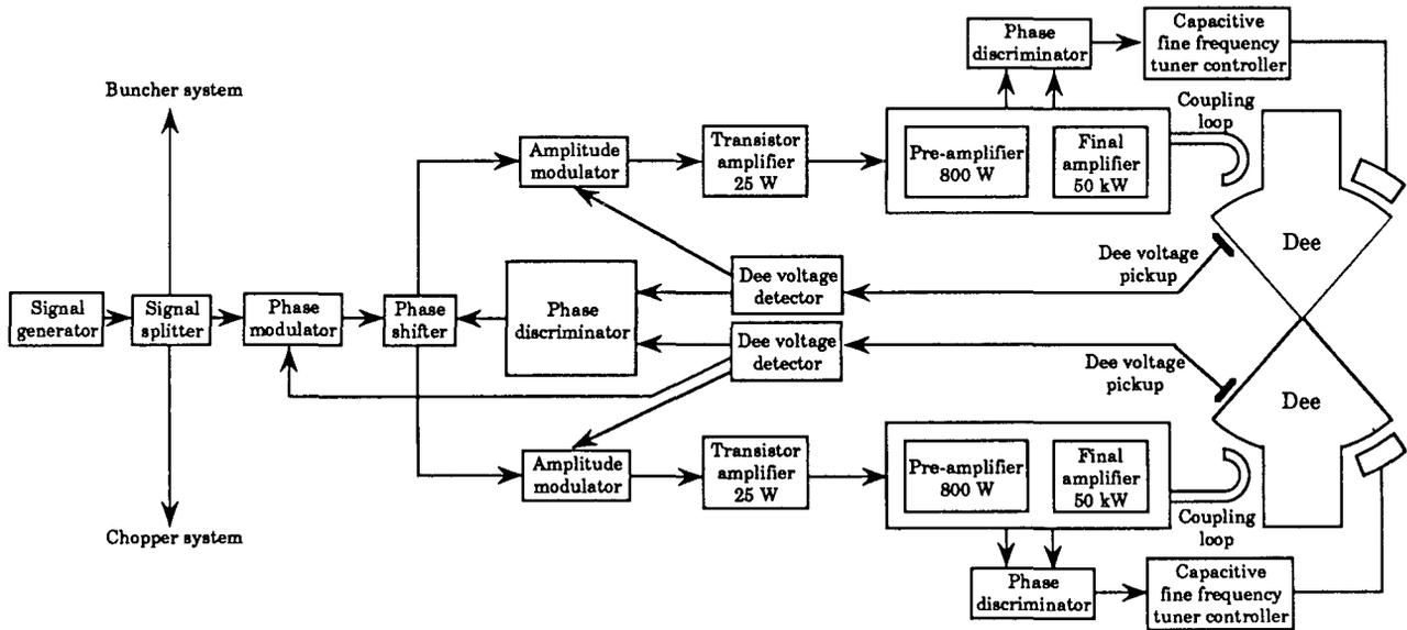
Fig. 8. Block diagram of the rf control system.
