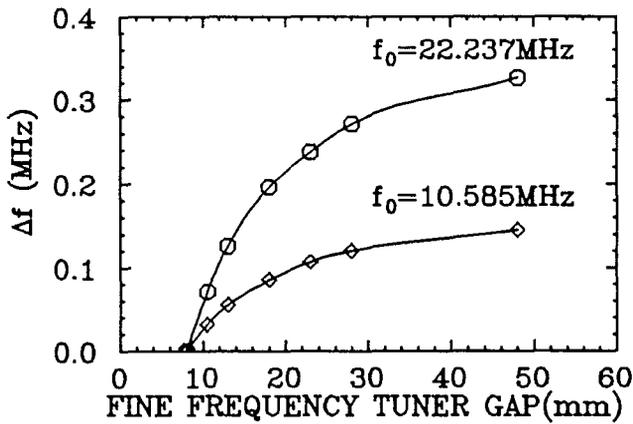
Fig. 4. Adjustable frequency by the capacitive tuner at 22.237 MHz and 10.585 MHz. The full relative frequency change is 1.6 %.
