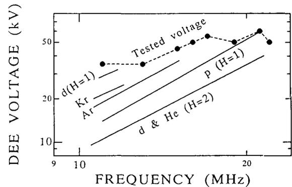
Fig. 9. The required dee voltage and tested voltage as a function of frequency.
