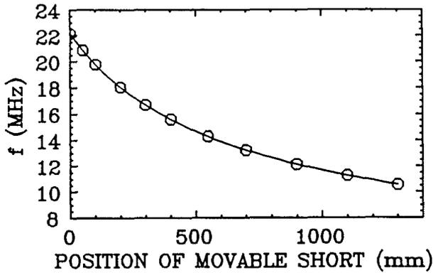
Fig. 3. Resonant frequencies of the resonator as a function of position of the movable shorting plate.
