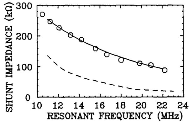
Fig. 6. Frequency dependence of shunt impedance. The solid line shows 75 % of the calculated value based on one-dimensional transmission line approximation. The dashed line shows the measured value of the movable panel type cavity.
