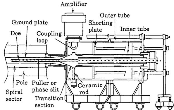
Fig. 2. Schematic view of the coaxial resonator with a movable shorting plate.
