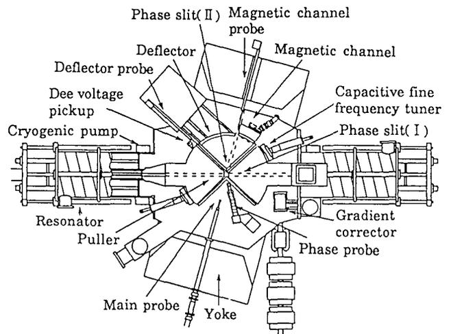
Fig. 1. Schematic drawing of the AVF cyclotron.
