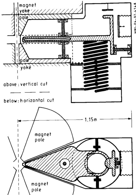
Fig. 1. Quarter wave resonator with helical inner conductor
