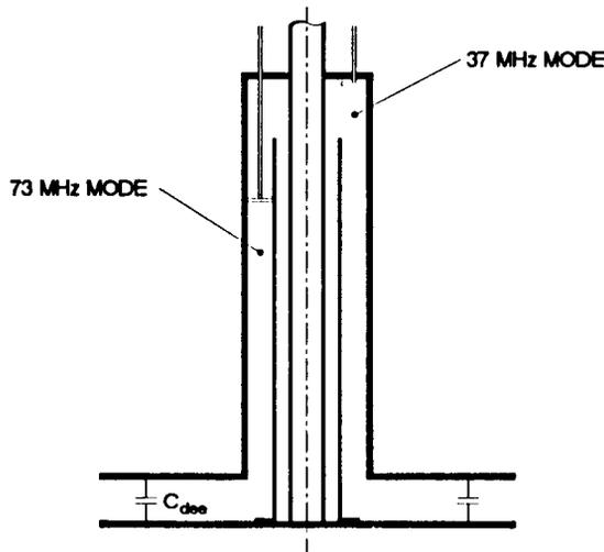
Fig. 5. Low loss folded cavity.
