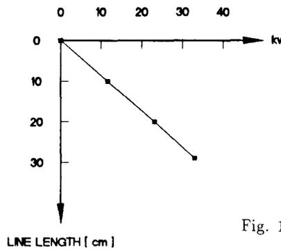
Fig. 10. Voltage measured along stem.
