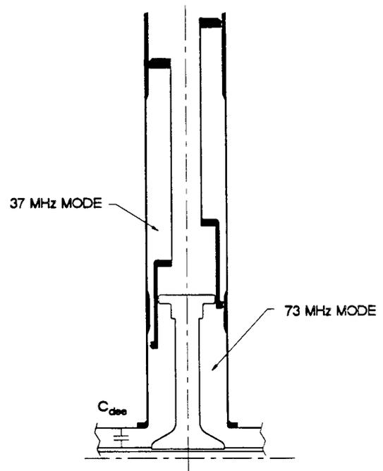
Fig. 6. Solution using a coaxial switch.
