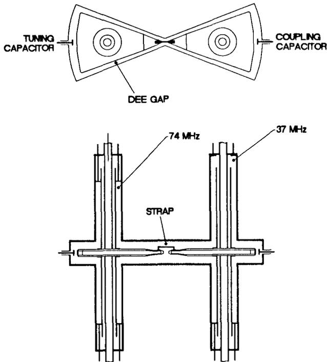
Fig. 2. Schematic diagram of the dual frequency resonator system.
