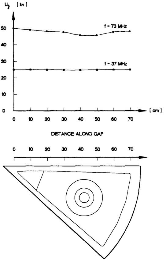
Fig. 9. Voltage measured at dee gap.
