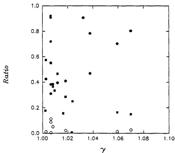
Fig. 4. The ratio of the current measured on the plate ILC04 to that measured on ILC02 (solid circles). The ratio of the beam measured at 26.5" to that measured on ILC04 (open circles). The ratio of the beam extracted from the cyclotron to that measured at the cyclotron extraction radius (solid squares). (Cf. paragraph 4)
