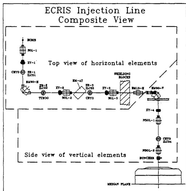
Fig. 3. The injection line components.
