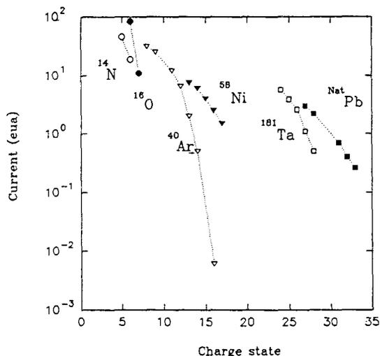
Fig. 2. Typical extracted currents for several ions ranging from  $^{14}\text{N}^{3+}$  to  $^{\text{Nat}}\text{Pb}^{33+}$  measured on a plate intercepting the beam after the analysis magnet (ILC02).
