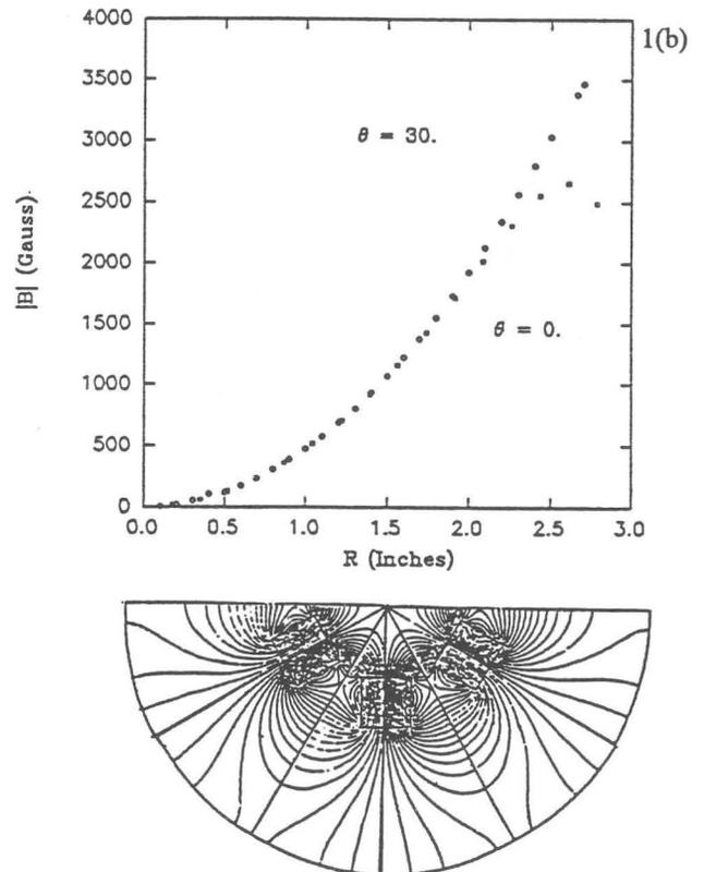
Fig. 1. A sketch of the principal elements of the magnetic structure and the associated field profiles. (a) The mirror field. (b) The hexapole field. The radius of the plasma chamber is at 2.5".
