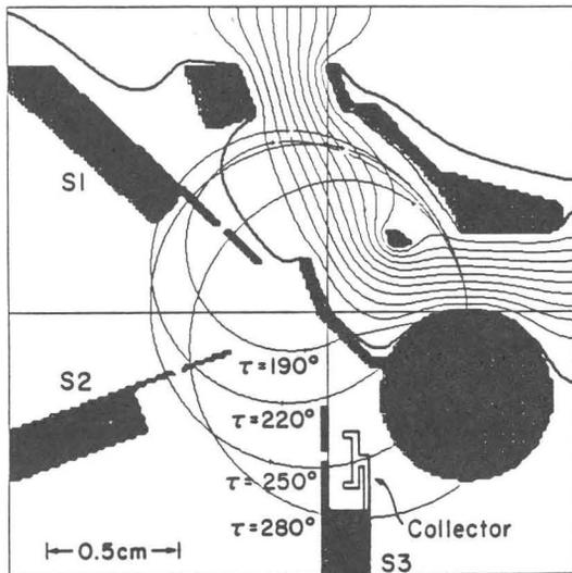
Fig. 2. The orbits on the schematic view are shown, calculated for 4 different rf phases ( $270^\circ$  is peak voltage on the first gap). The initial energy of  $D^+$  is 250 eV, and ions are started at the center of the source with zero divergence angle.
