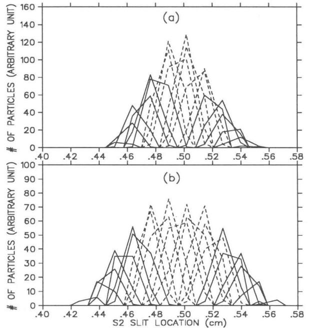
Fig. 6. The current distributions simulating the measurement are calculated for the initial conditions in the second and third lines of Table 1. The individual curves are obtained at different S1 locations as slit S2 is scanned. (a) has 19 curves(0.191 cm wide spread in S1 coordinate) , while (b) has 24 curves(0.267 cm wide spread).
