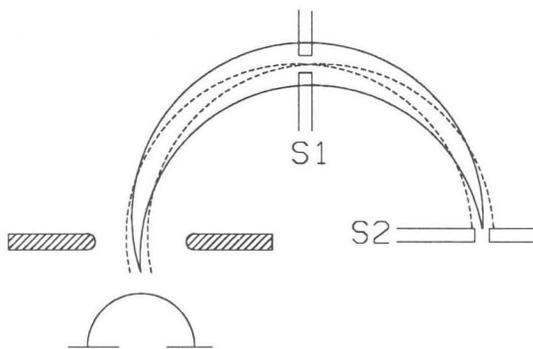
Fig. 5. The usual two slit method in the dc experiment.<sup>3)</sup> The slit S1 selects the divergence, and the slit S2 scans the beam size. The S3 in our central region functions similar to S2 as initial divergence becomes less sensitive, while the beam spreads well by phase difference.
