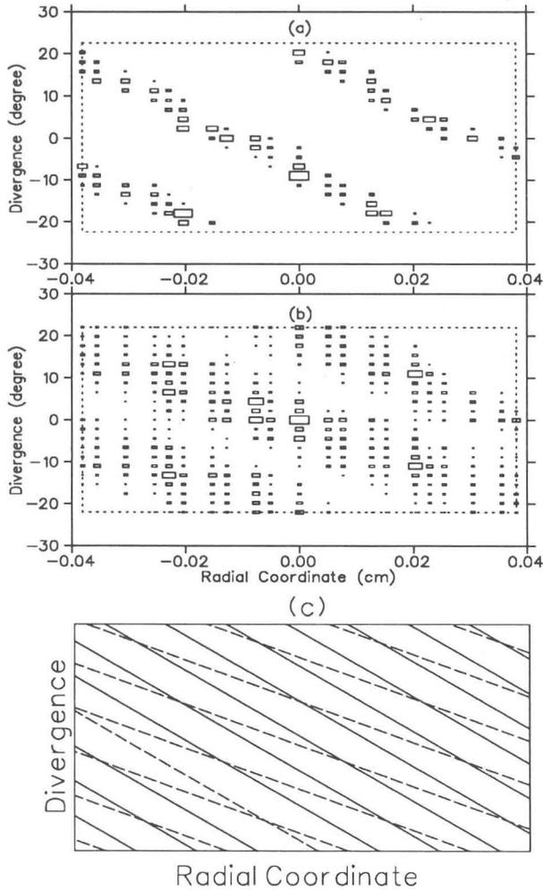
Fig. 7. The source phase space selected by slit S1 and S2 of 0.05 mm wide. The initial condition is same as the second line of Table 1 and with S3 fixed selecting  $\tau$  around  $215^\circ - 225^\circ$ . The three separated regions in each figure correspond to three different locations of S1 in (a), and S2 in (b) with the other slit scanned, respectively. (c) shows the sketch of pixels selected by both slits.
