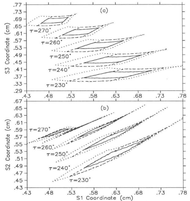
Fig. 3. The projection of the rectangular initial phase space into the slit coordinate space for five different rf starting time in the interval of 10 degrees. The dashed line is for a larger source width, and the dotted line is for an increased divergence angle, which are described in Table 1. The area occupied in the slit coordinate space shrinks for the same emittance as the rf starting time rises.
