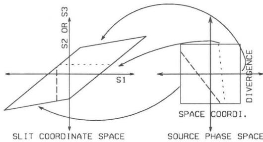
Fig. 4. Sketch of the transformation of boundaries from source emittance to slit coordinate space, The rectangular shape is deformed to a parallelogram.
