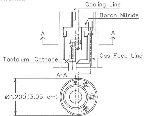
Fig. 1. PIG source designed to fit on the central hole of 8-Tesla magnet
