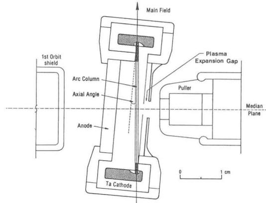
Fig. 1. A rotation mechanism to adjust the value of the expansion gap.
