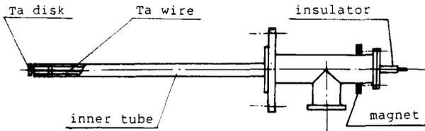
Fig.10. The cold cathode for CAPRICE.
