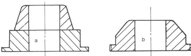
Fig.2. The shape of original ring (a) and new ring (b)
