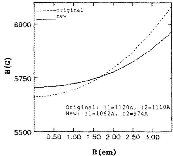
Fig.8. Magnetic field vs radius near the extraction.
