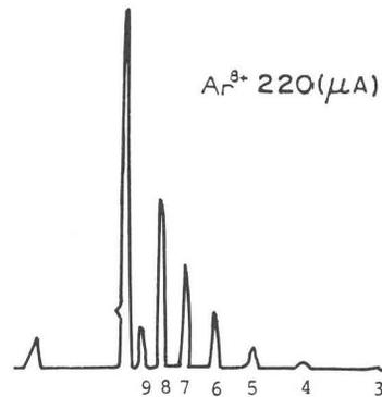
Fig.4. Ion spectrum optimized for  $Ar^{8+}$ .
