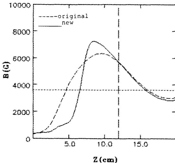
Fig.7. Axis magnetic field near the extraction. Original:  $I_1 = 1120.A, I_2 = 1110.A$ . New:  $I_1 = 1062.A, I_2 = 974.A$
