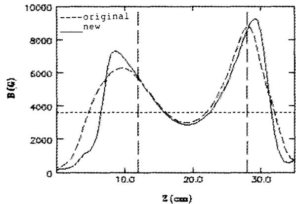
Fig.9. The final  $B$  along source axis after change. Original:  $I_1 = 1120.A, I_2 = 1110.A$ . New:  $I_1 = 1062.A, I_2 = 974.A$
