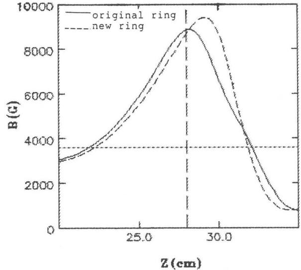
Fig.3. Magnetic field  $B$  along source axis. Coil current  $I_1 = 1120.A, I_2 = 1110.A$ .
