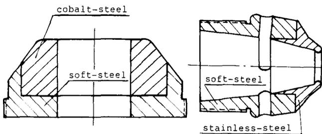
Fig.5. New conical ring with cobalt-steel.
