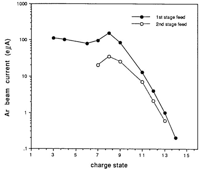
Fig. 1 Charge distribution of Ar ions, comparing 1st and 2nd stage feeding of Ar gas.
