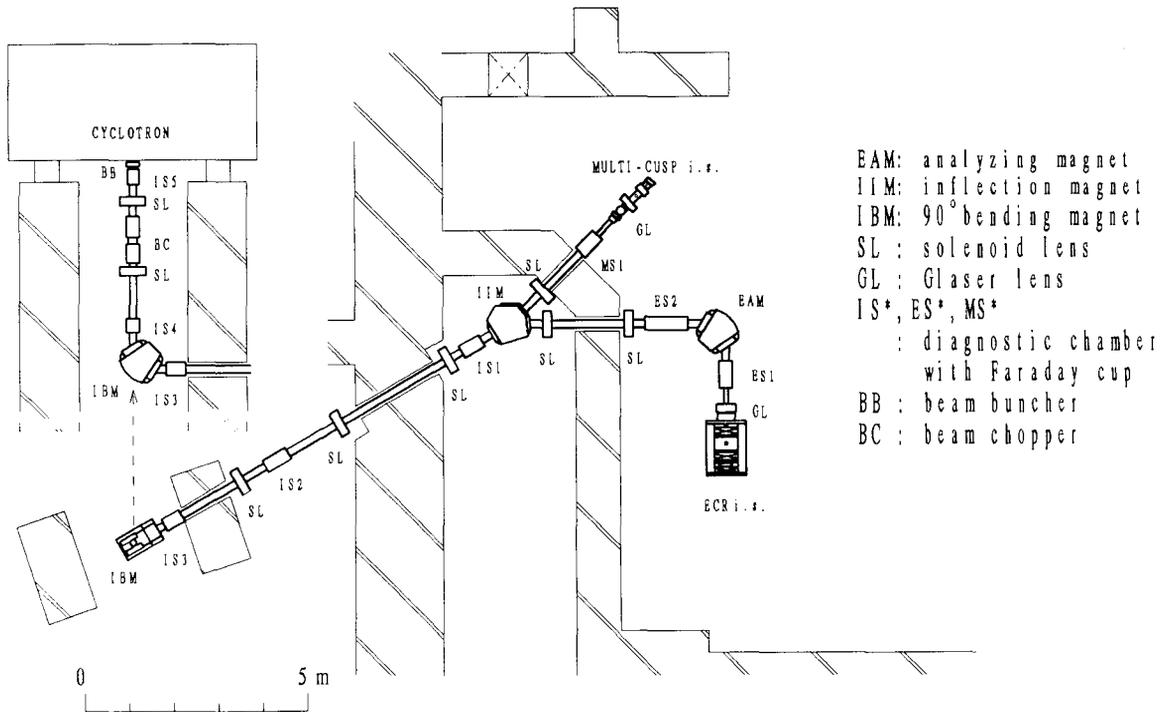
Fig. 3 Schematic layout of the ion sources and the injection line.
