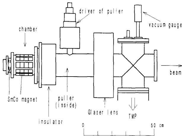
Fig. 2 Side view of the multi-cusp ion source.
