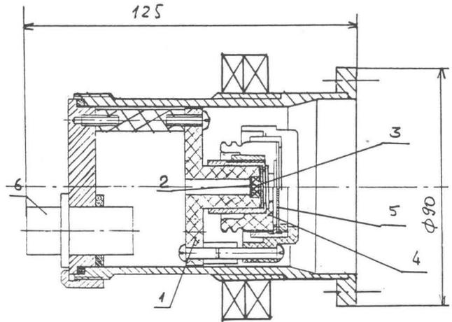
Figure 1: Ion source section
