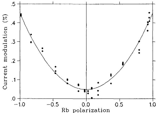
Fig. 8. Modulation of  $H^-$  current between polarized and unpolarized conditions, as a function of Rb polarization. The data were taken at a Rb thickness of  $4 \times 10^{13}$  atoms  $cm^{-2}$ . The polarization was varied by adjusting the frequency tune of the pumping lasers. The curve is a least squares fit to the data of  $CM = a + bP^2$ , where  $a$  and  $b$  are adjustable parameters. The standard error of  $b$  is  $\pm 1.0 \times 10^{-4}$ .
