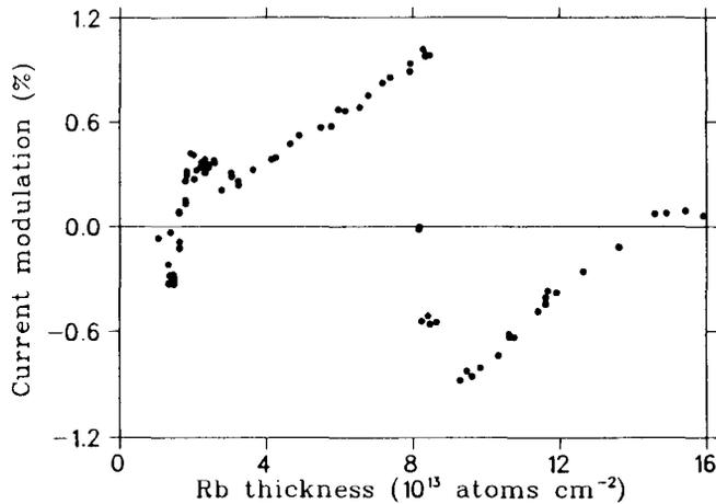
Fig. 7. Modulation of  $H^-$  source current between unpolarized and polarized conditions, as a function of Rb thickness.
