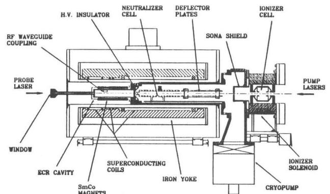
Fig. 1. Schematic diagram of the TRIUMF optically-pumped polarized H<sup>-</sup> ion source.
