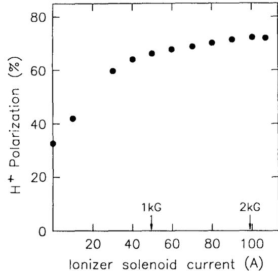
Fig. 6. Proton polarization dependence on ionizer-cell magnetic field.
