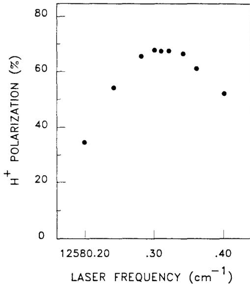
Fig. 4. Proton polarization as a function of pump laser frequency, for a single 5 W laser having a bandwidth (FWHM) of  $0.1 \text{ cm}^{-1}$ . The laser frequency was measured with a Burleigh WA-10 wavemeter.
