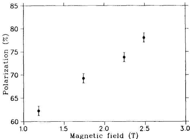
Fig. 5. Proton polarization as a function of magnetic field in the Rb cell.
