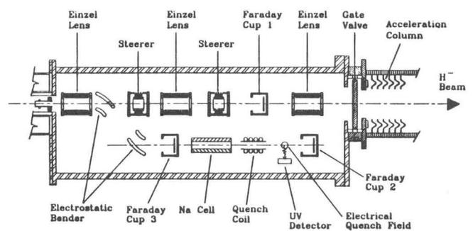
Fig. 2. Schematic diagram of the beam transport optics downstream of the ion source, and the Lyman-α polarimeter contained within the same chamber. During normal source operation the H<sup>-</sup> beam passes through a 2.0 cm diameter aperture in the first electrostatic bender. During polarimeter operation deflecting voltages are applied to the benders. Faraday Cups 1 and 3 can be moved out of the beam axis. The UV detector is a dual microchannel plate protected by a LiF window.
