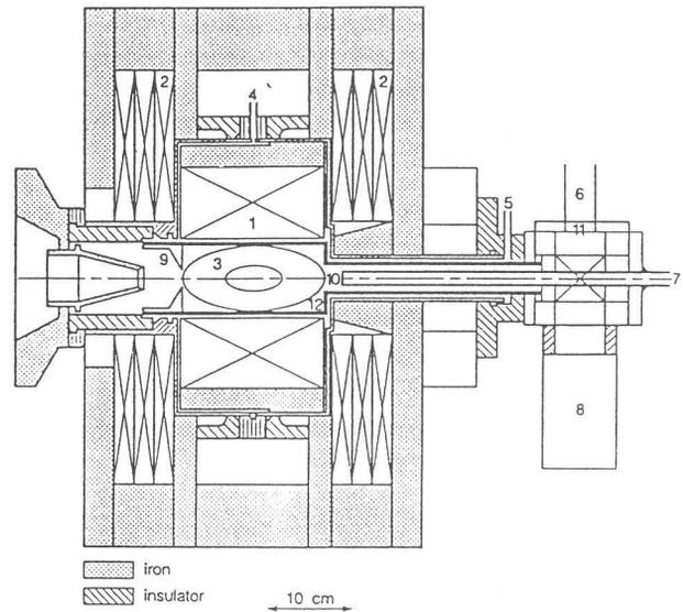
Fig. 1. Elevation view of the CAPRICE- $2\omega_{ce}$  source. (1) shows the sextupole magnet. (2) shows the solenoid magnets. (3) shows an inner ellipse where the ECR resonance condition is met. On the outer ellipse the magnetic field is twice as great. (6) shows RF waveguide which feeds into a transition section. (10) shows the end of the coaxial coupling.
