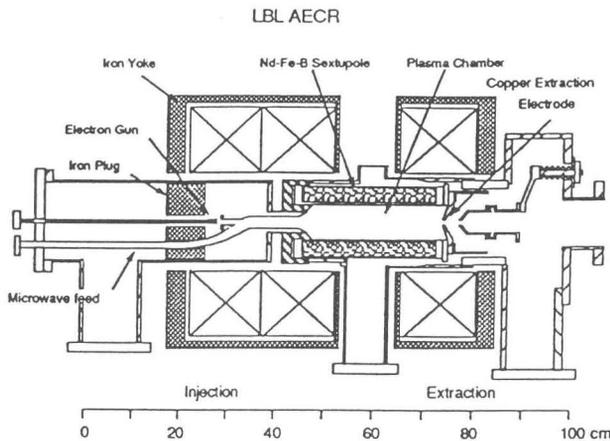
Fig. 2. Elevation view of the LBL AECR. This Nd-Fe-B sextupole has radial slots for pumping the plasma chamber. RF power is fed by a transition from rectangular to round waveguide.
